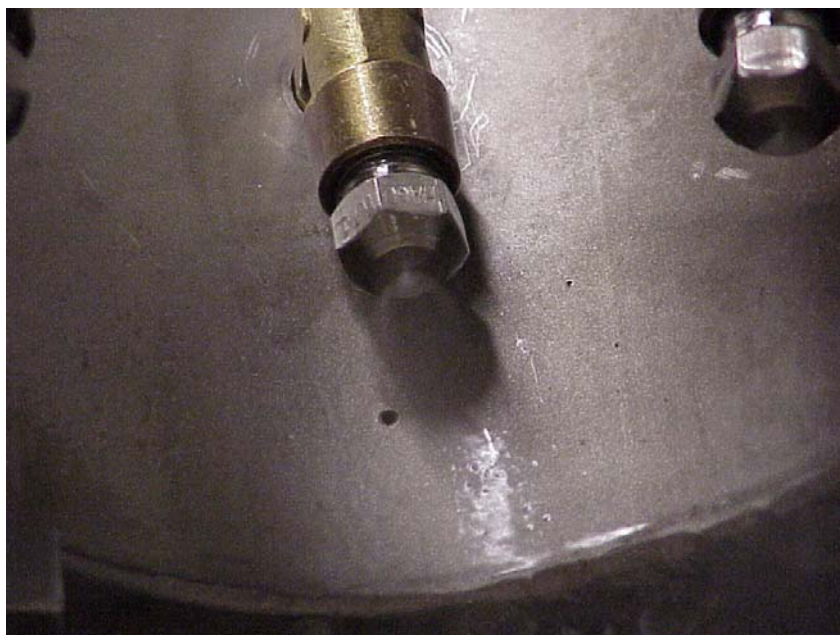
Figure 18. Fuel Spray from M1 Injectors at 20 psi (detail)
