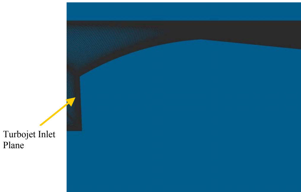
Figure 49. Detail of first grid without any grid points inside the turbojet engine
