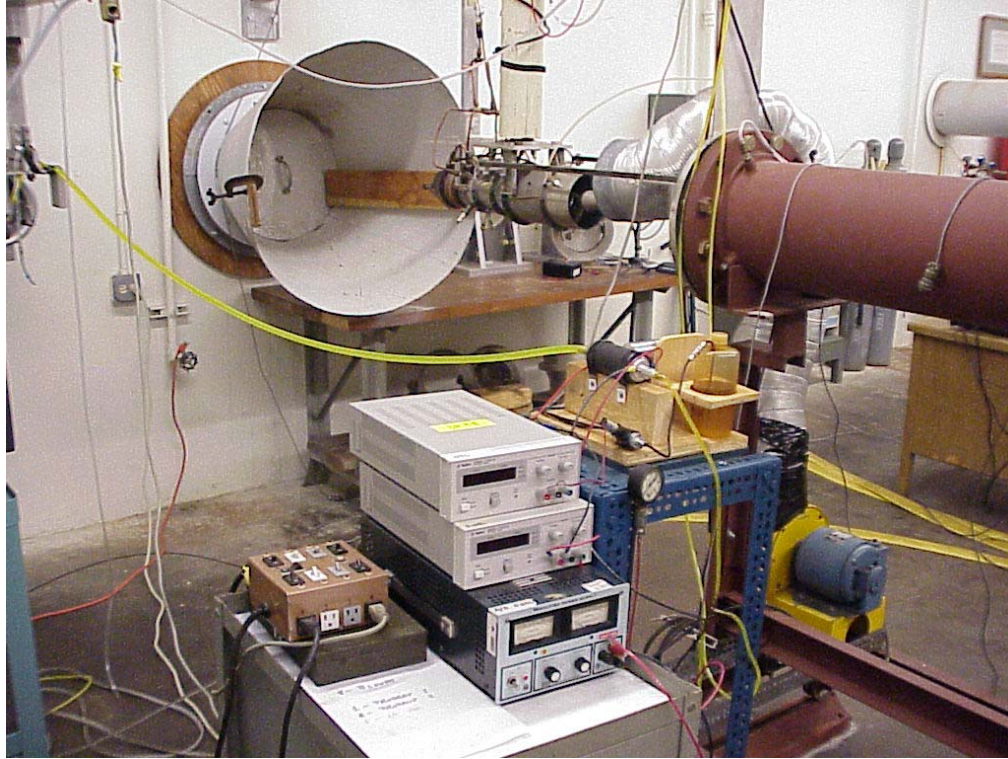
Figure 3. Engine Test Rig and Controls
