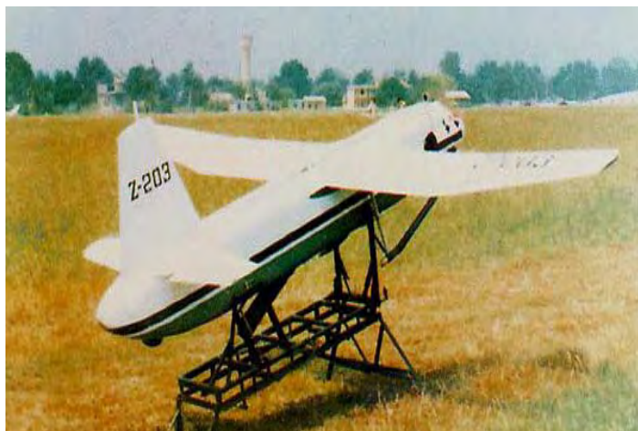
UAV uses a reusable solid rocket booster prior to jettison after take off
