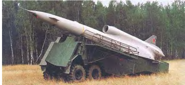
Tu-243 on launcher vehicle
