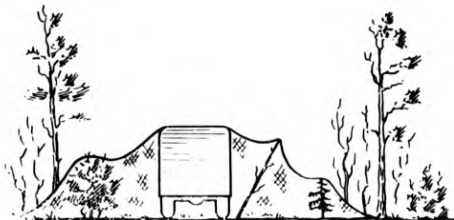
Figure 30. Shape of a screen cover when camouflaging equipment in a sparse forest.
