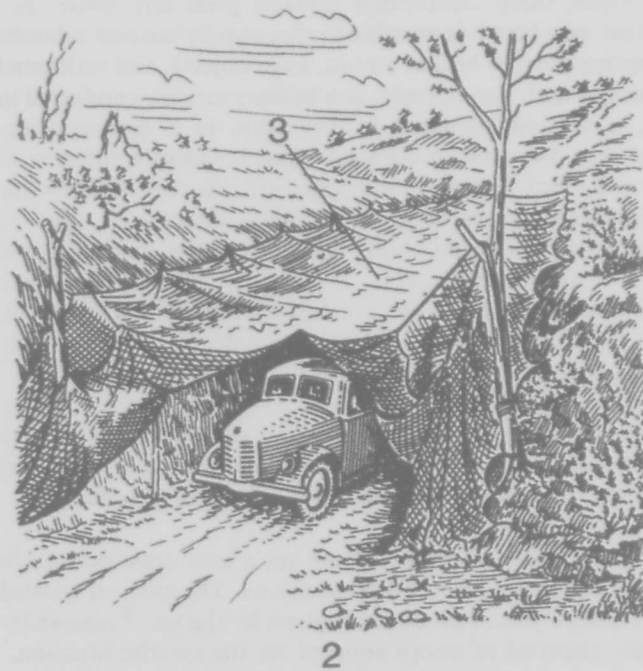
Figure 32. Methods of camouflaging equipment in a ravine.
