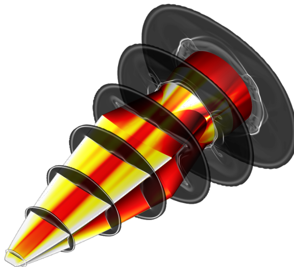
Figure 13. Example JHU/APL BOLT II mean flow results, showing surface heating in orange, and numerical schlieren in grayscale.
