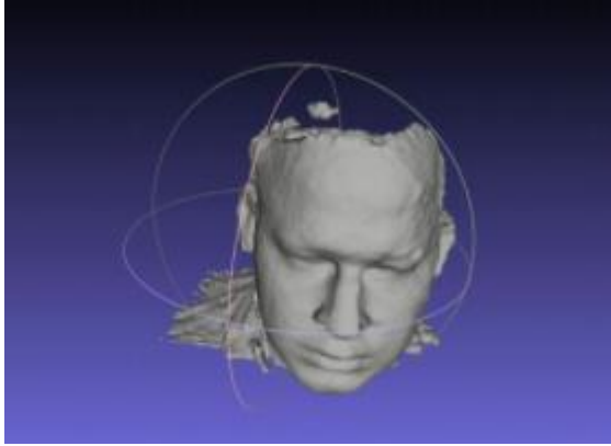
Fig 6: A 3d mesh of a student's face using the Structure.io sensor.
