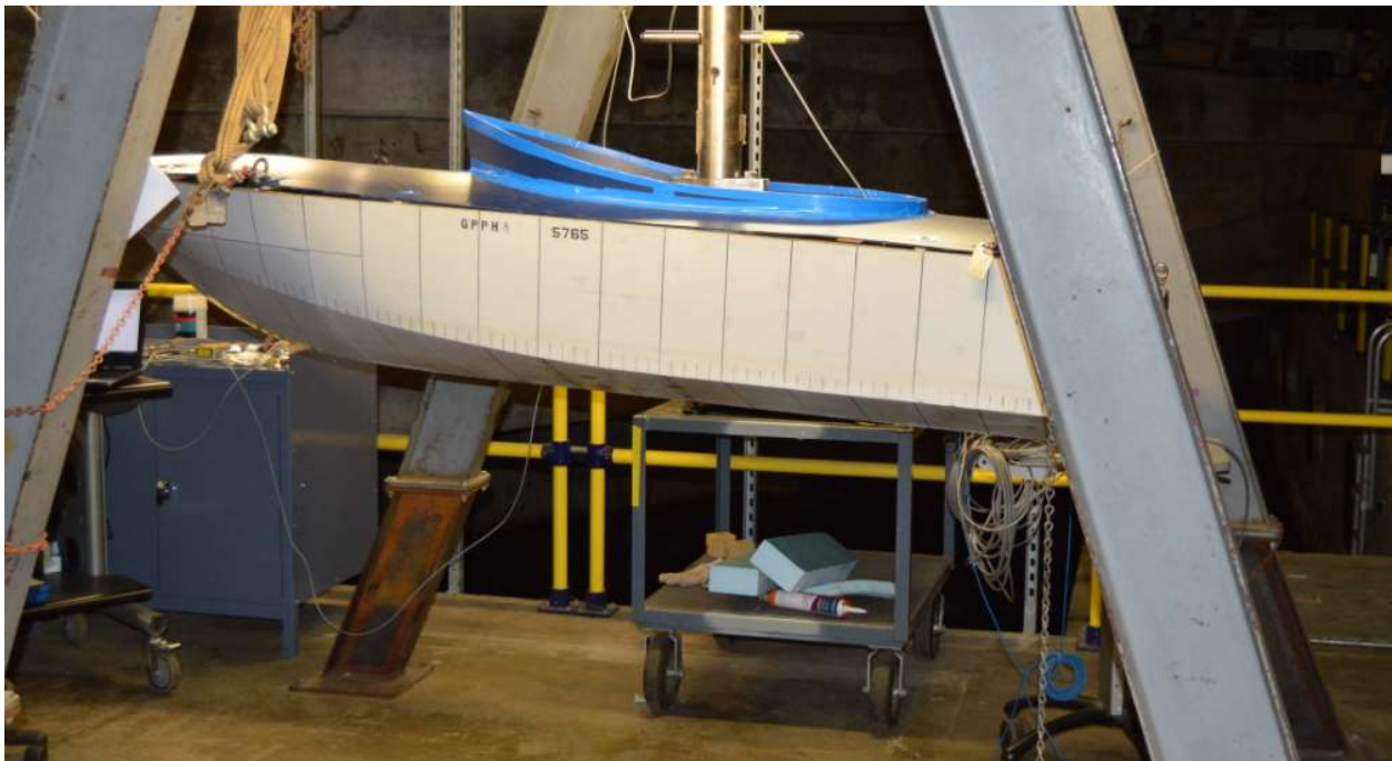
Figure 19. Model Suspended from A-Frame During Ballasting
