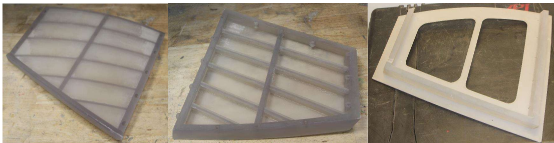
Figure 14. Traditional Grillage and Backing Plate Made from Accura60
