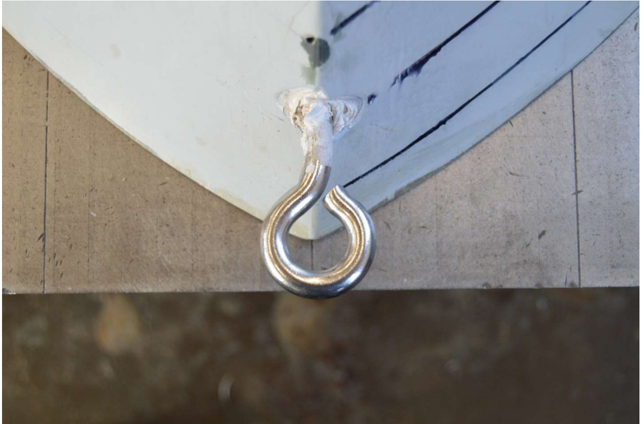
Figure 5. Stem Aligned with Marking on Steel Table
