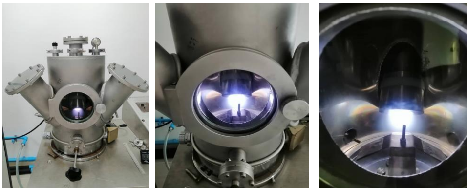
Figure7. The process of the formation of nanoparticles over the surface of PBS/E1/PBAT/MgO composite film by DC magnetron sputter coating method.
