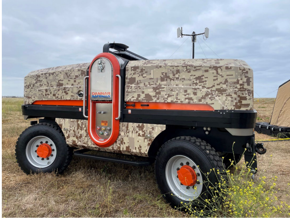
Figure ES-2. DANNAR MPS powering the deployed AWS ICE payload during testing at Camp Pendleton.
