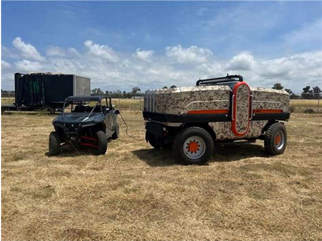
Figure 2. The DANNAR MPS charging a Volcon tactical EV.
