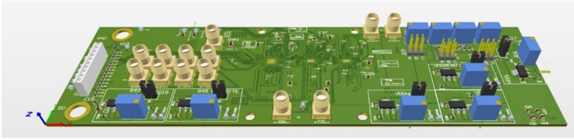
Figure 16 - 3D Render of the Final MRAM PCB Design
