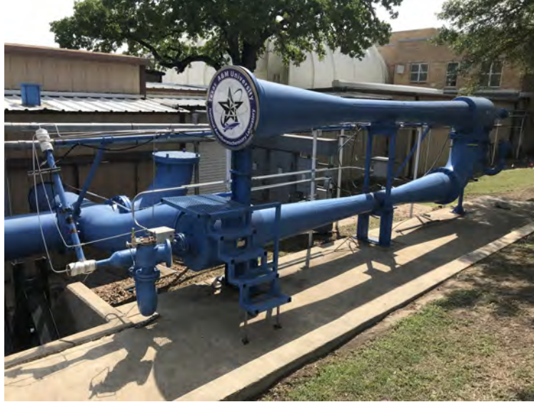
Figure 4.1: The two-stage air ejector.
