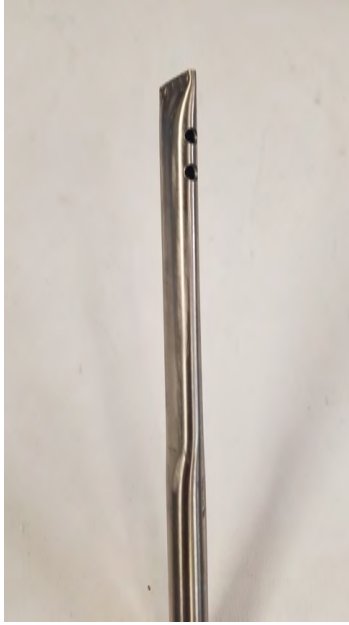
Figure 4.4: A characteristic NO seeder.
