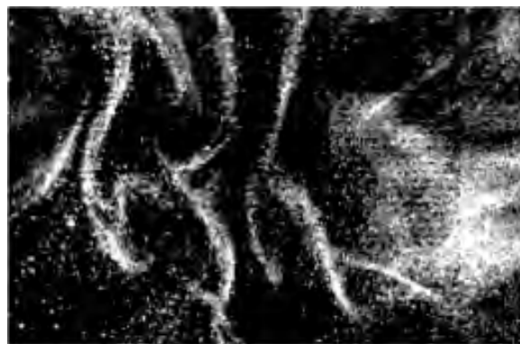
Figure 4.32: Mie scattering image of diaphragm debris from run 67. [11].
