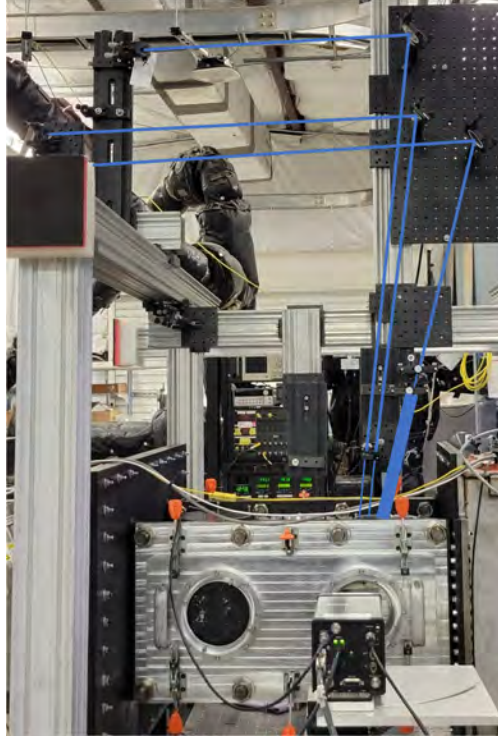
Figure 6.14: PLIF MTV setup. Two "Write" lines are used to double the usable data. [7]
