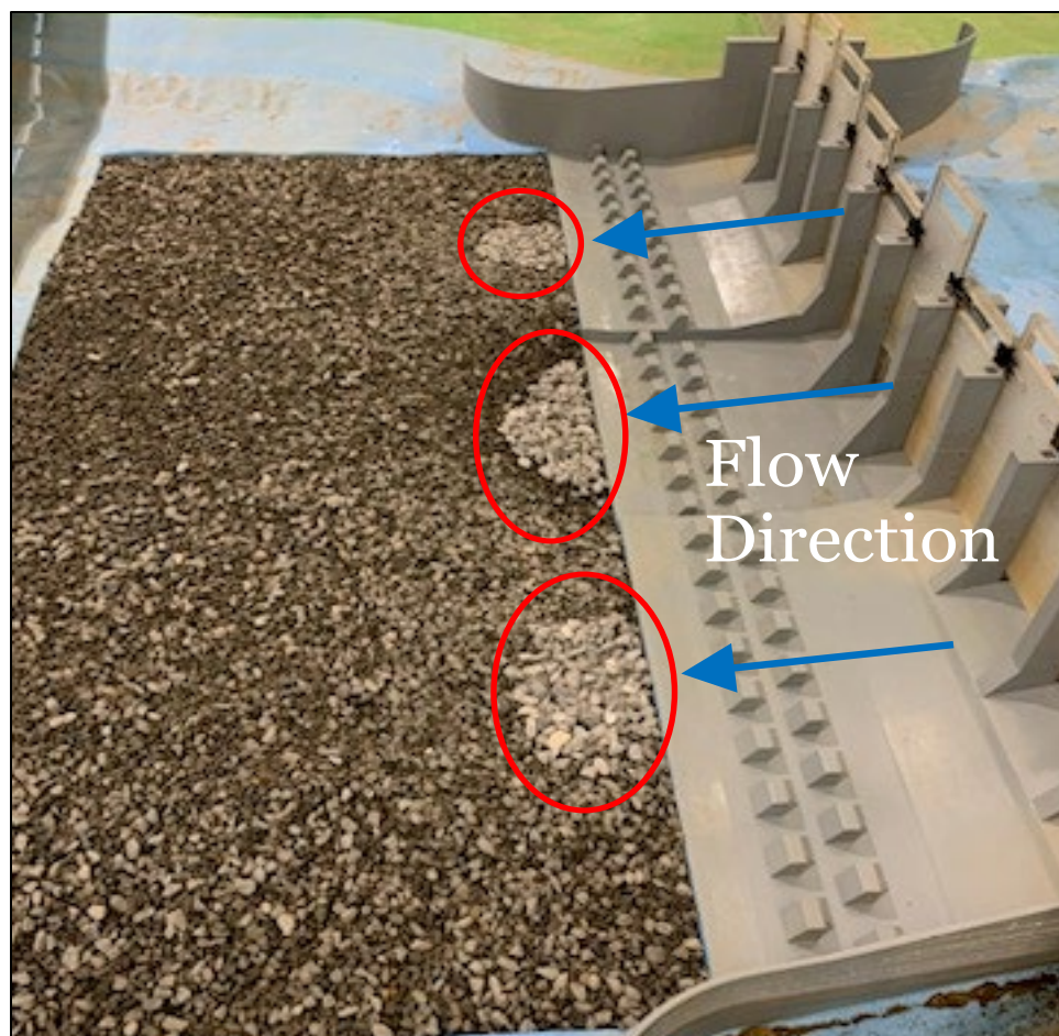
Figure 27. Scour holes filled with Gradation B stone.
