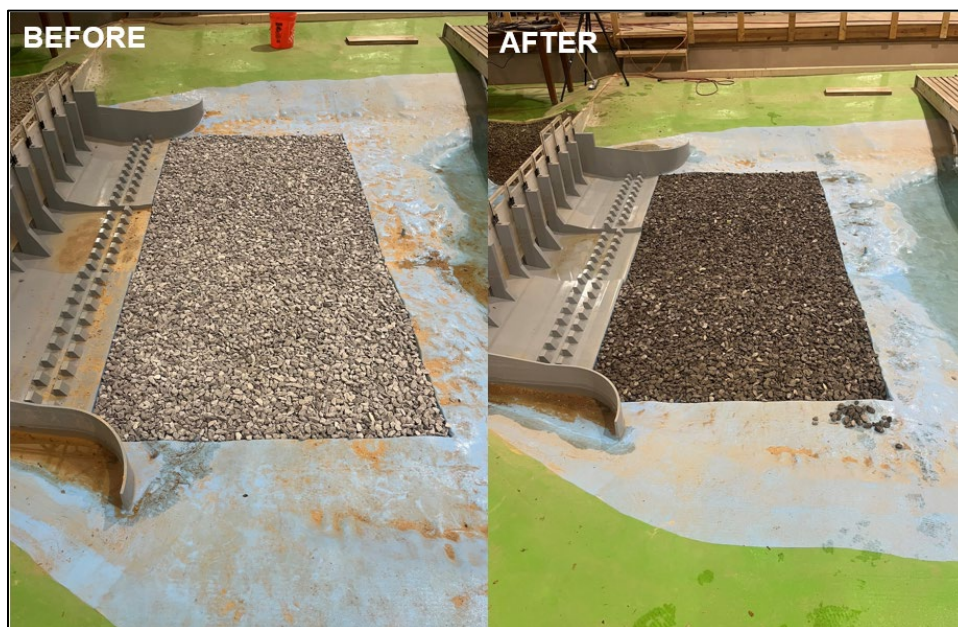
Figure 22. Before and after testing of Gradation B.
