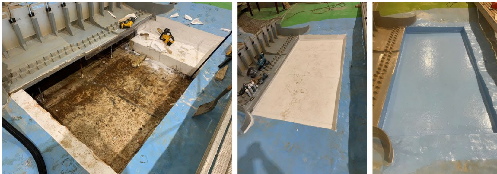
Figure 5. Model modifications: initial removal of existing blocks ( left ), new lowered blocks placed and sealed ( middle ), and final area painted with polyurea ( right ).
