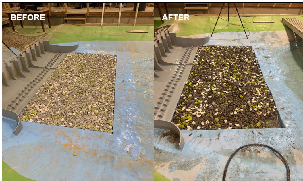
Figure 17. Photograph of Gradation A test area before and after testing.
