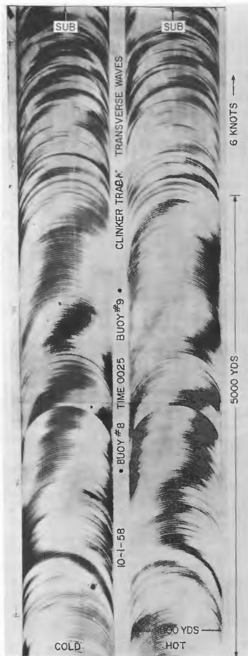
Chart 4 - Scar from USS NAUTILUS underway at 6 knots at a keel depth of 200 ft on edge of hurricane Helene. Apparent jaggedness in the scar is due to motion of airship. Transverse waves at the top are bunched together due to airship pitching.
