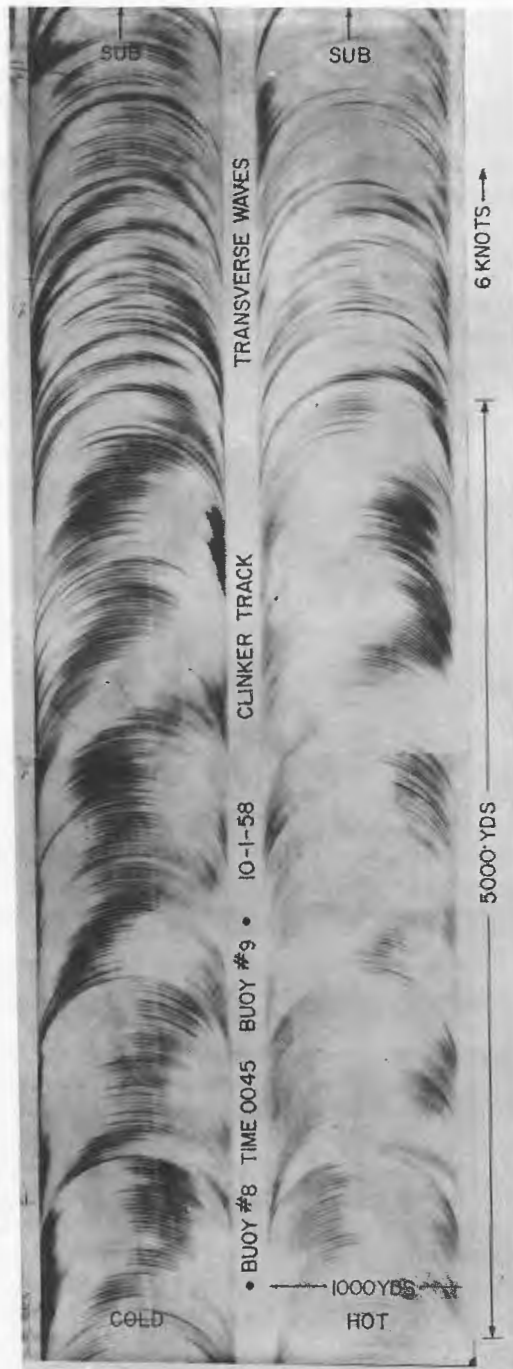
Chart 5 - Second recording made 20 min after that of Chart 3, showing scars behind USS NAUTILUS while underway at 6 knots and a keel depth of 200 ft (unclass)
