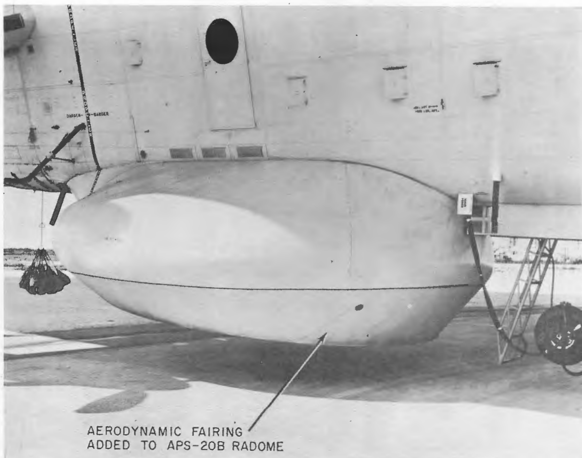
Fig. 70 - Aerodynamic fairing added to existing APS-20B radome for AN/AAR-23(XB-1) installation (Unclassified)
