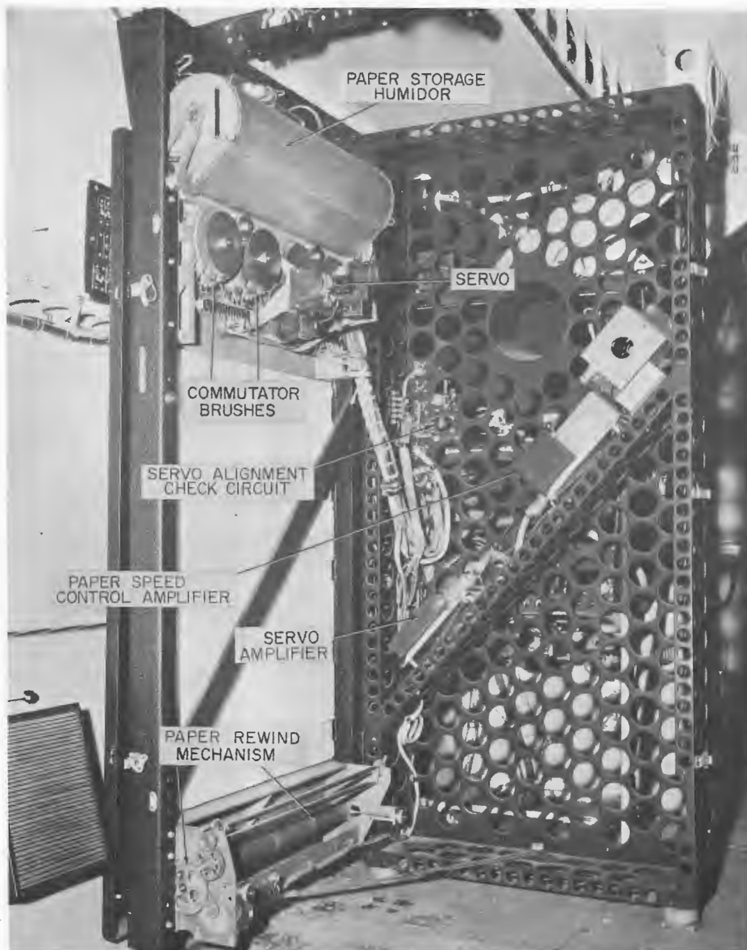
Fig. 51 - Interior of three-coordinate mapper
