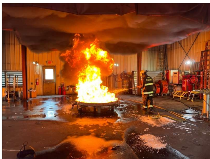
Figure 2: Ignited fuel in 28 sq ft pan and application of foam-additive mixture.
