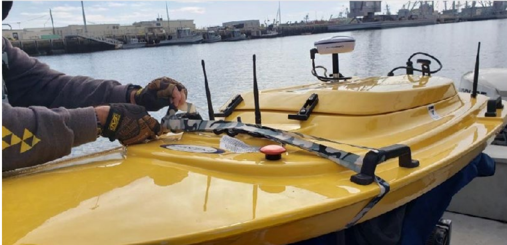
Figure B-17. Detail showing threading the straps through the front handles on the Z-boat and tightening with the ratchet.
