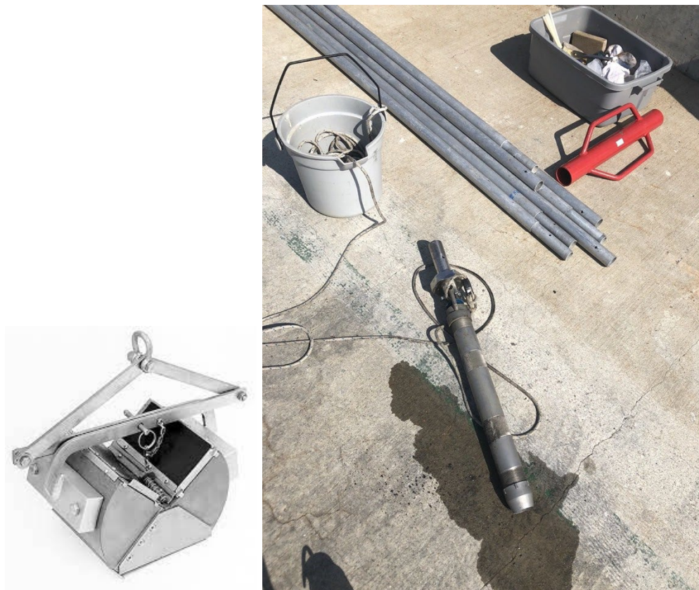
Figure 15: (Left) Mini ponar sampler used to collect grab-samples of surface sediments under piers and (right) Manual coring system used to collect push-cores up to 24 inches long under piers.
