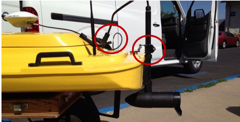
Figure B-3. Detail showing how to plug propeller cable into the receptacle in the boat hull.
