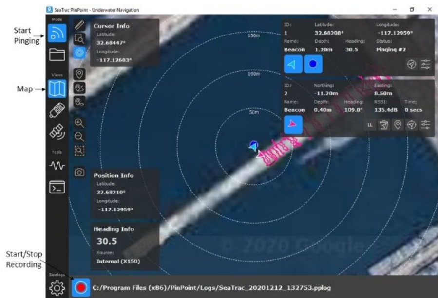
Figure 5. Diagram of the SeaTrac ultra-short baseline acoustic “diver tracker” system used to estimate the coordinates of the Z-boat when it was in the GPS-denied environment under the piers.
