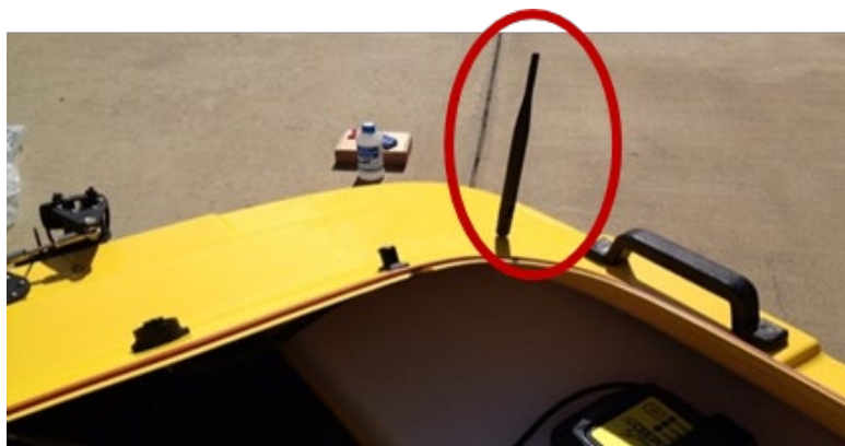
Figure B-5. Detail showing one female omni-directional antenna in left rear receptacle.
