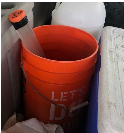
Figure B-55. Example of a capped and labelled core positioned upright in a bucket. Blue ice packs surround the lower portion of the core to keep it cold.
