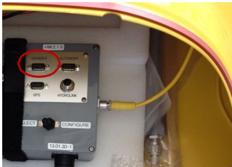
Figure B-9. Detail of the “Sounder” port to which the CEEPULSE echosounder power/data cable must be connected.
