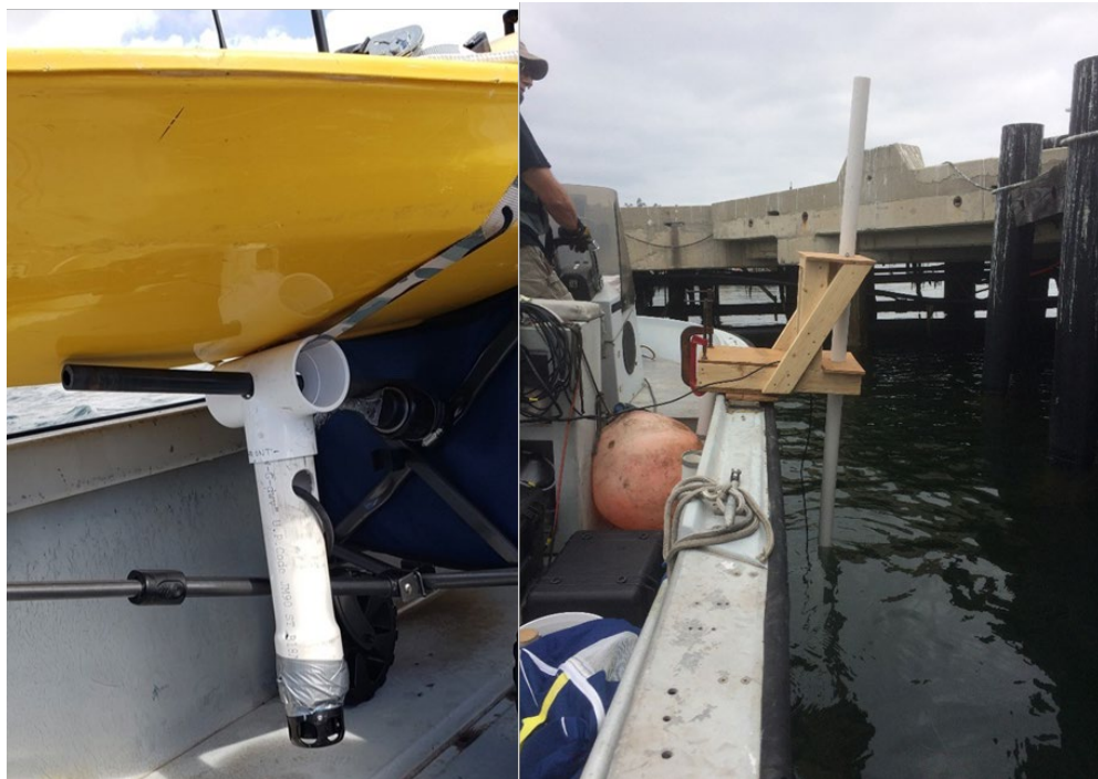
- Mounting system for USBL beacon on Z-boat (left) mounting system for topside USBL beacon (right).
