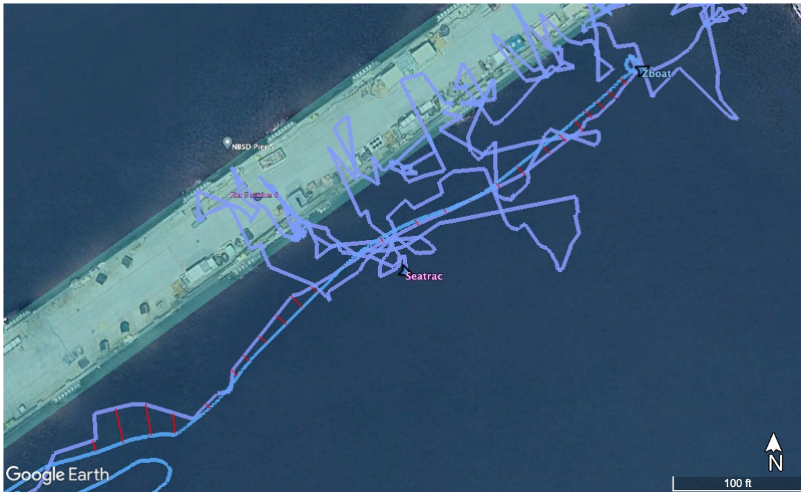
Figure 18. Z-boat positions recorded by the integrated GPS (blue) and SeaTrac system (purple) for one of the Pier 5 surveys, with locations where the difference between positions was measured for a track along the length of the pier indicated with red lines.
