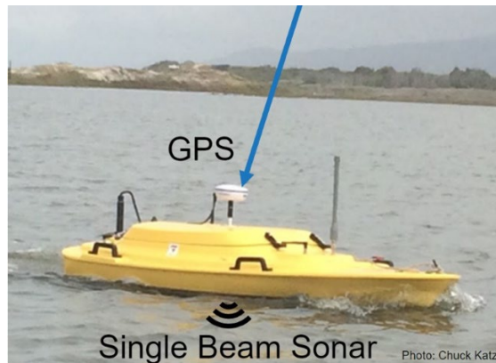
Figure 3. Z-boat used for bathymetric mapping under pier areas.
