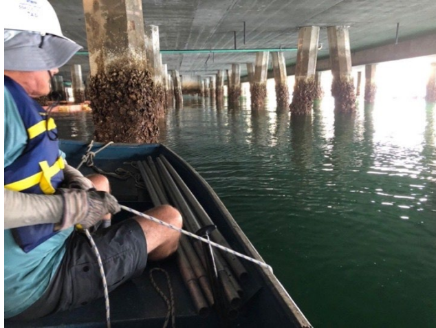
Figure B-52. A member of the under-pier team lowers the grab sampler over the side of the workboat using a line.
