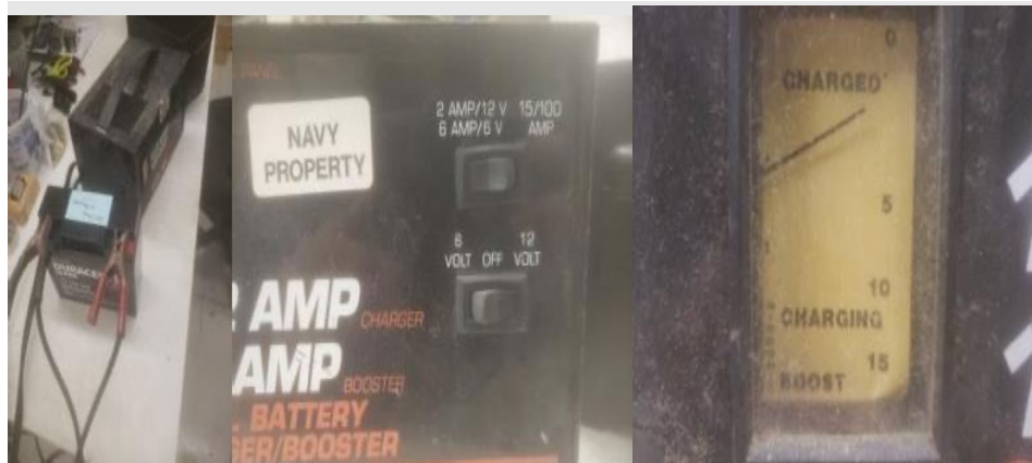
Figure B-1. Marine battery being charged (left). Settings for battery charger (middle). Battery charge indicator (right).
