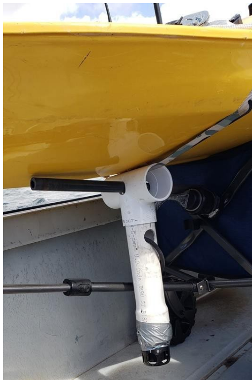
Figure B-18. Z-boat beacon mounting system, with the gray stabilizing arms of the mount facing the bow and stern.
