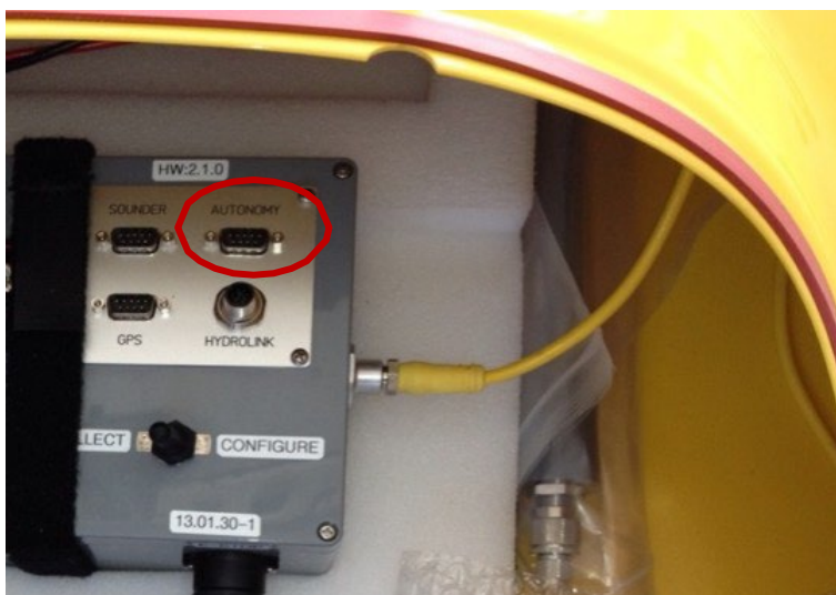
Figure B-11. Autonomy port highlighted in red, to which the data cable from the compass must be connected.
