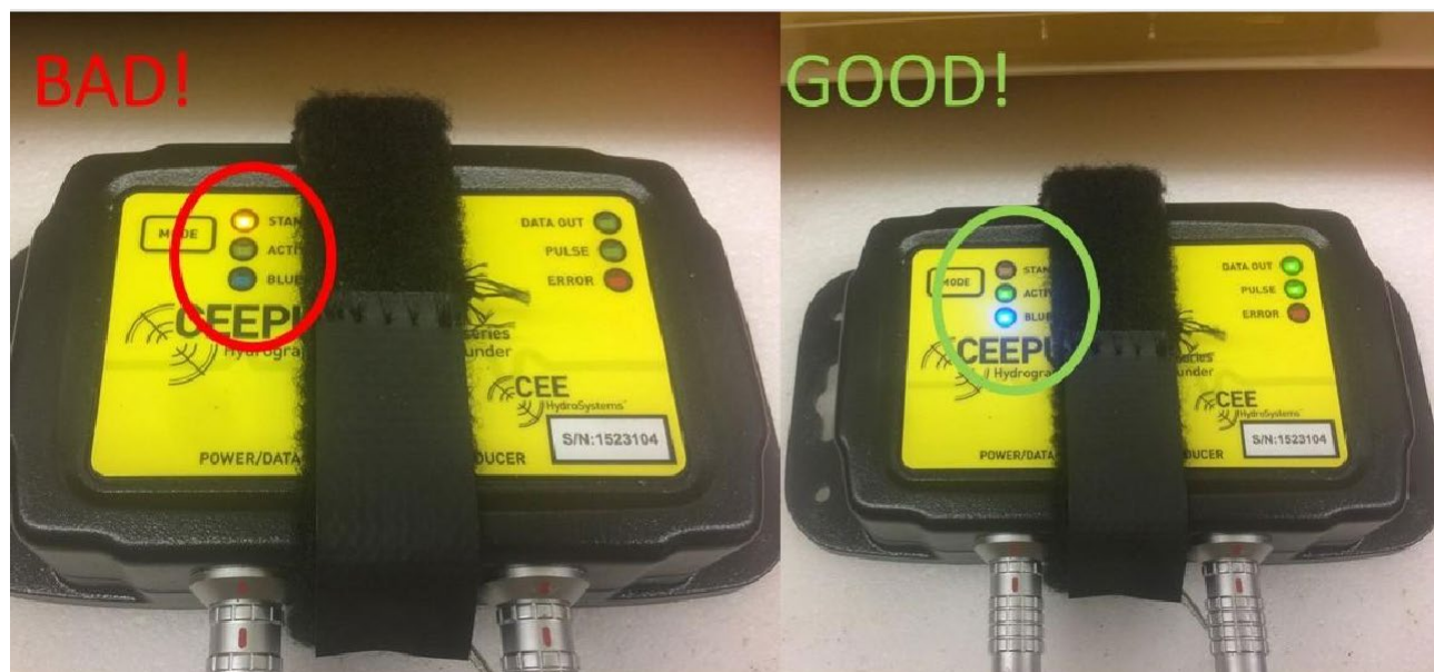
Figure B-24. CEEPulse light configurations: good and bad examples shown.
