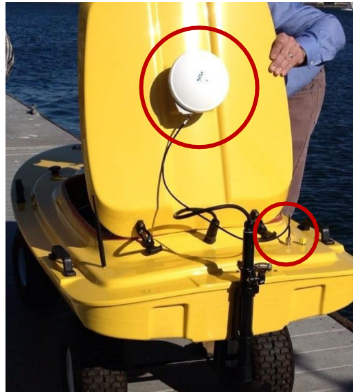
Figure B-12. White GPS antenna attached to the top of the boat hatch, with the GPS cable connected to the antenna and rear right port.
