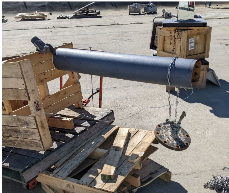
Figure 75. Loaded Frangible Bolt Coupler Test
