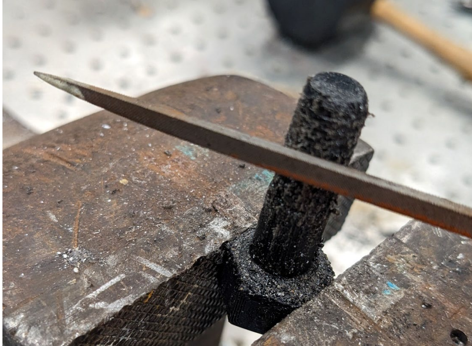
Figure 85. Cleaning Frangible Bolt with Triangular File
