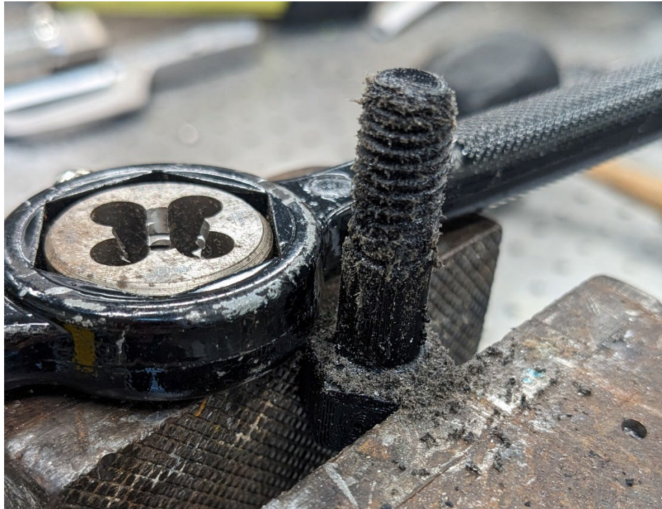
Figure 86. Bolt Threads After Chasing
