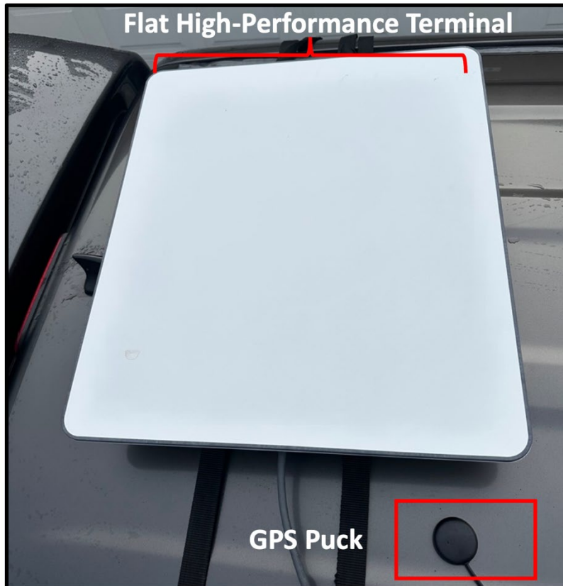
Figure 23. Starlink Mobile Test Setup
