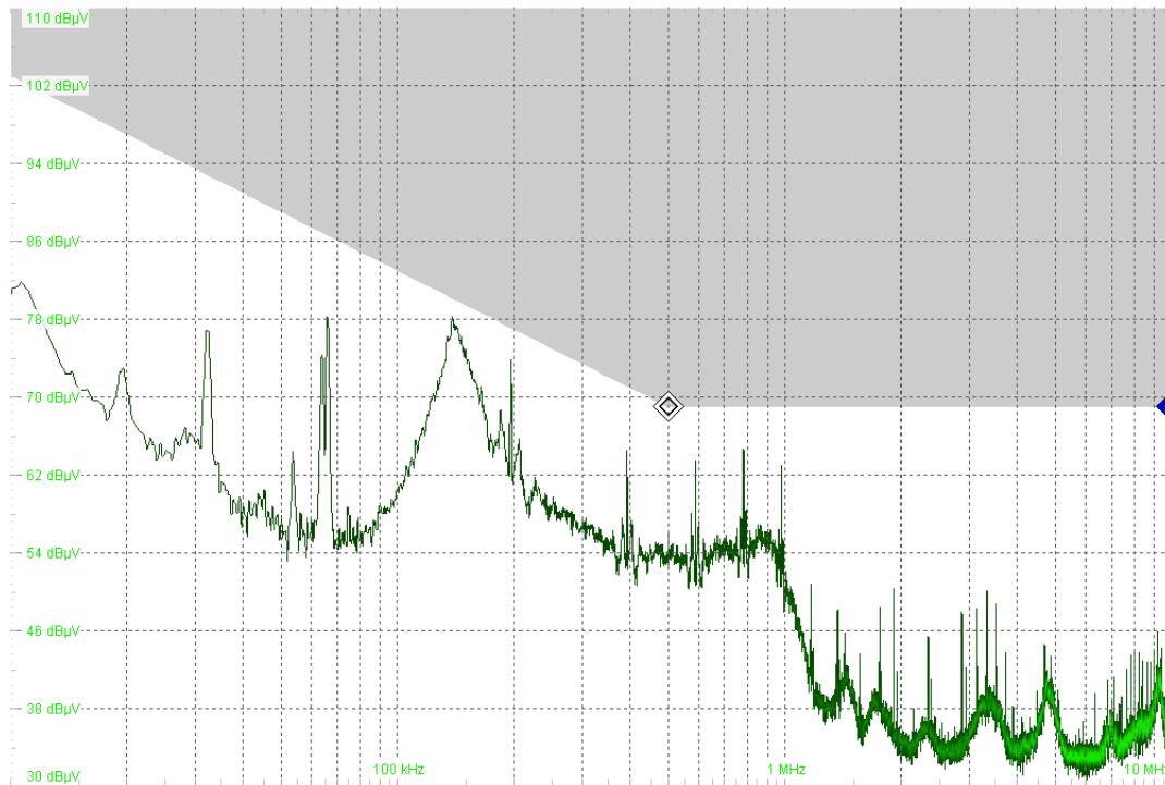
Figure 6.7. CE 102 compliance for 300 ns dead-time, 6.8 nF bypass capacitor, and with compensation method on.
