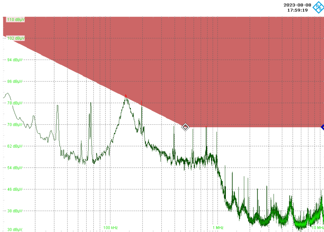
Figure 6.6. CE 102 compliance for 300 ns dead-time, 6.8 nf bypass capacitor, and with compensation method off.
