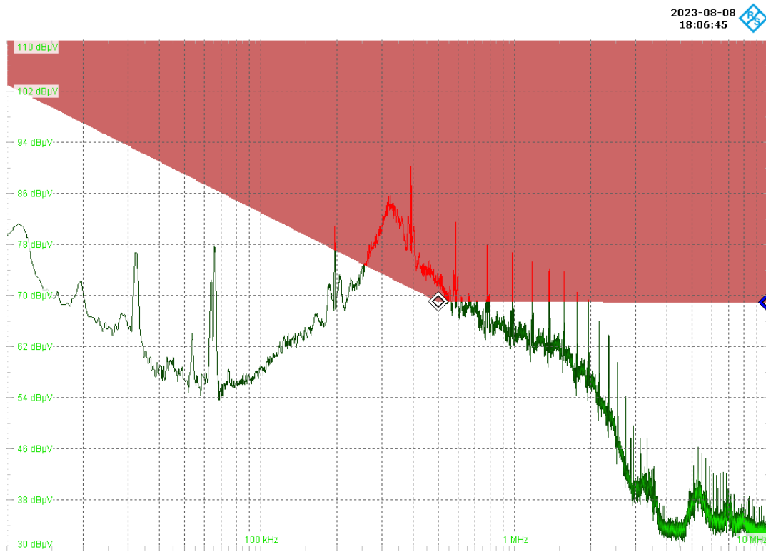
Figure 6.8. CE 102 compliance for 300 ns dead-time with compensation method off without a bypass capacitor.
