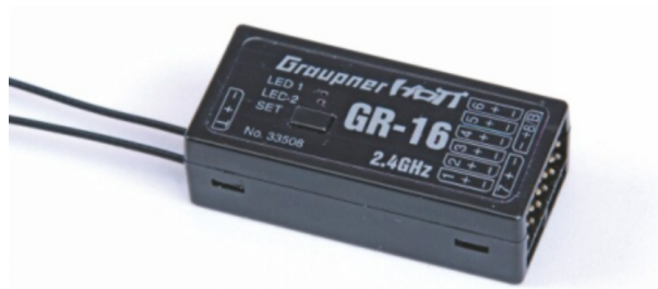
Figure 12. RC Radio Receiver (Model: Graupner GR-16 8CH 2.4GHz HoTT). Source: [13].
