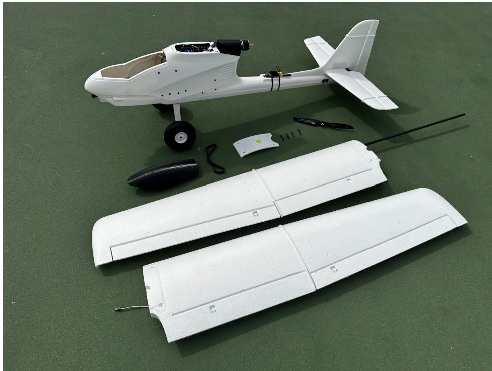
Figure 3. Photo of a Partially Disassembled SIM-1 UAS
