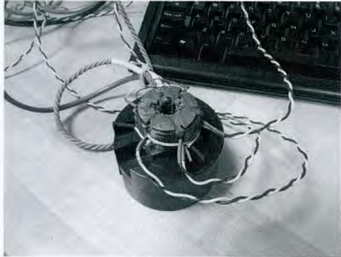
(b) Stator assembly
