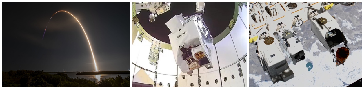
Figure 4. The CRS-27 nighttime launch on March 15, 2023. The removal of STP-H9 from the SpaceX Dragon trunk. STP-H9 (the middle payload) installed on the JEM-EF aboard the ISS.
