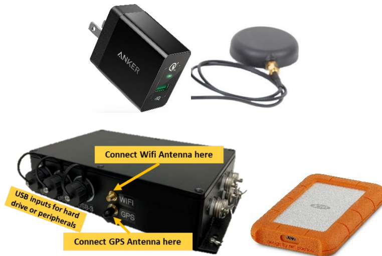
Fig. 3 Provided USB QC charging block (top left), GPS antenna (top right), view of MUGS connectors (bottom left), and rugged LaCie HDD (bottom right)
