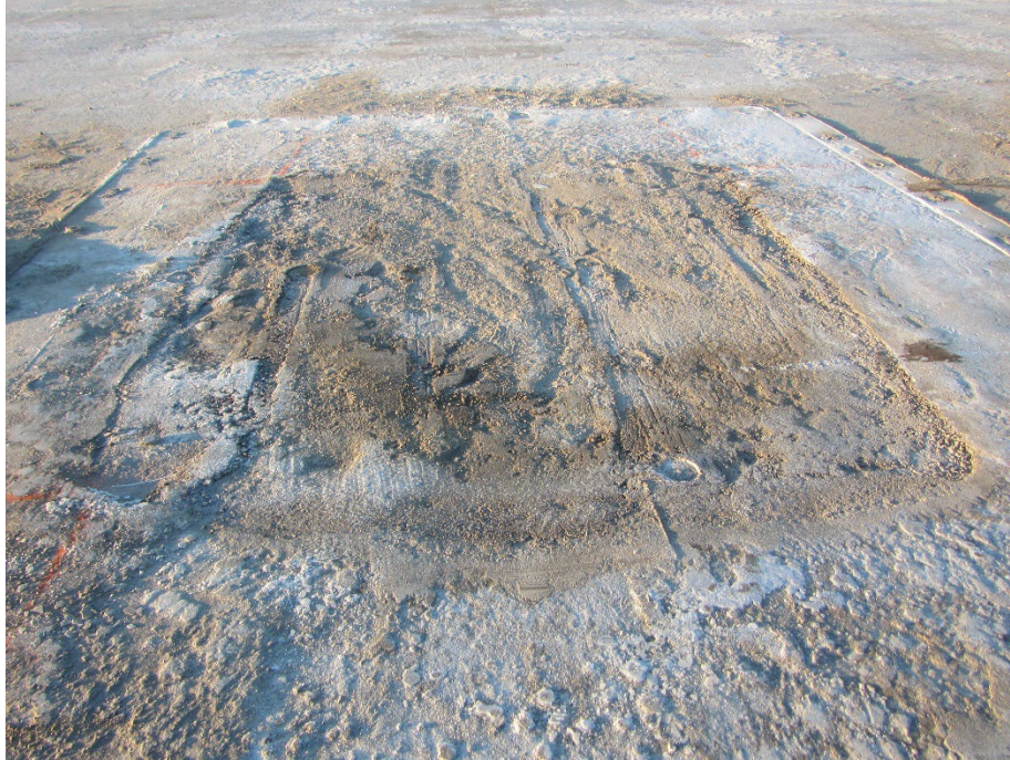
Figure 60. Repair 6, overall surface of RSFF backfill, 500 passes.
