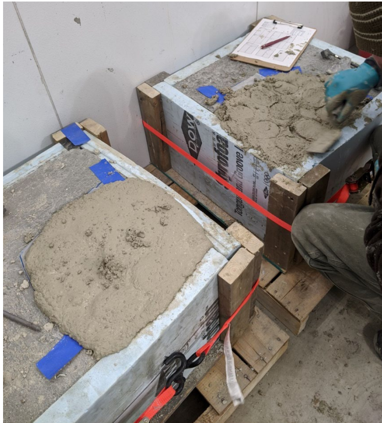
Figure 4. Troweling surface of specimens.
