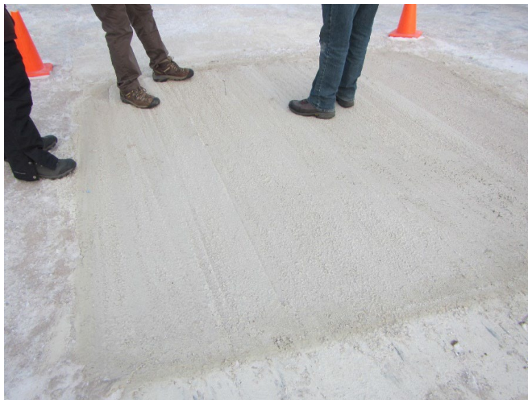
Figure 61. Repair 7, 12 hr cure time, 0 passes.
