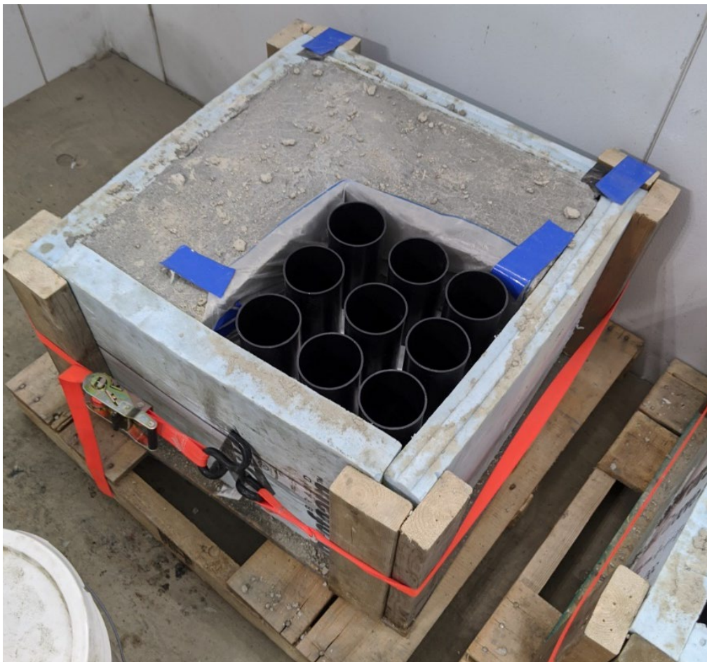
Figure 3. Fully assembled CARTS apparatus in the cold room, ready for testing.
