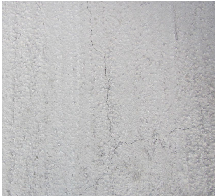
Figure 62. Small shrinkage cracking on Repair 7, 18 hr cure time, 0 passes.
