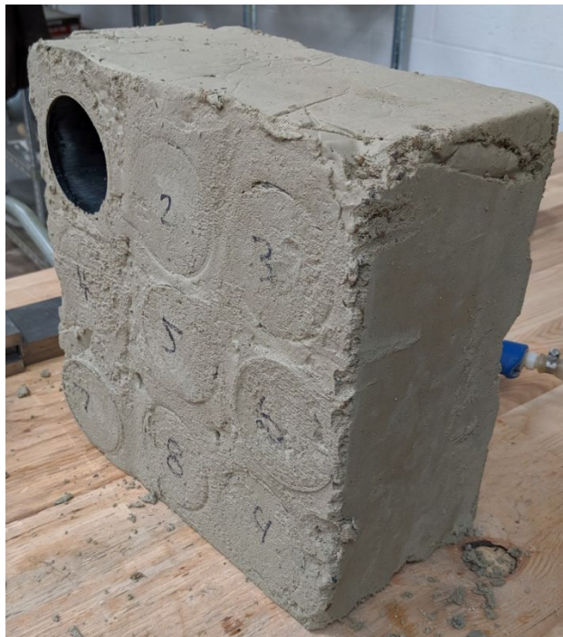
Figure 5. Removing specimens from the mold.
