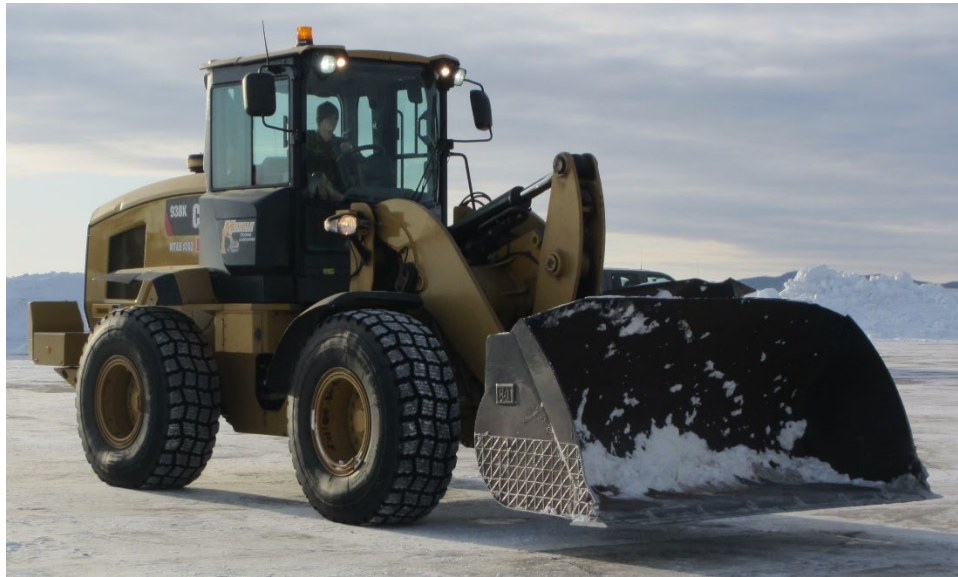
Figure 20. Caterpillar 938K front-end loader.
