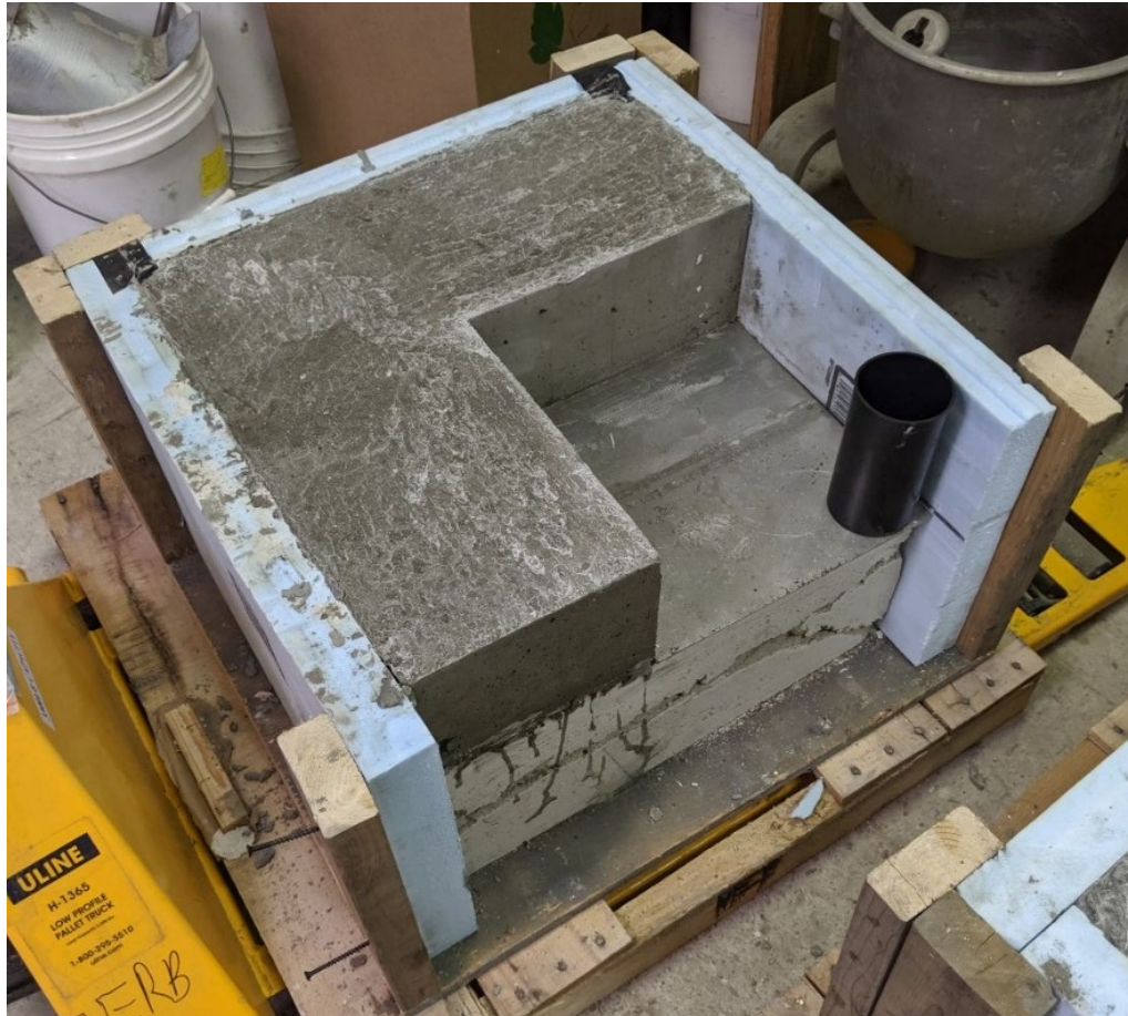
Figure 1. Concrete Airfield Repair Thermal Simulator (CARTS) apparatus with one side of the mold removed, showing a simulated patch area, and pallet jack underneath.
