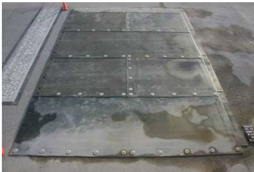
Figure 36. Assembled fiber-reinforced polyester (FRP) matting system.
