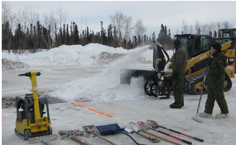
Figure 42. Processing stockpiled snow with snowblower attachment.
