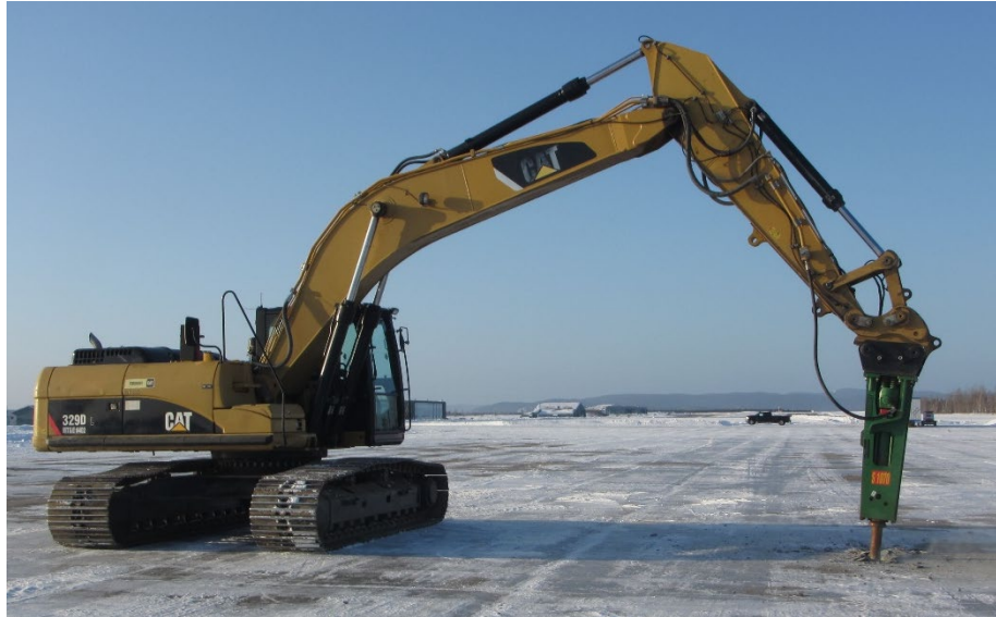
Figure 40. Pavement breaking with CAT 329D excavator.
