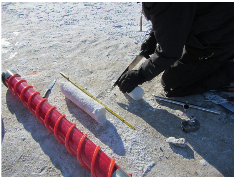
Figure 71. Core sectioning for weight and volume measurement to calculate density.
