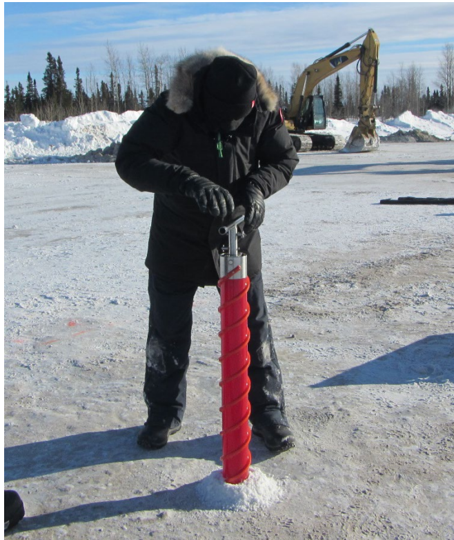
Figure 70. Core drilling compacted snow-water slurry sample.
