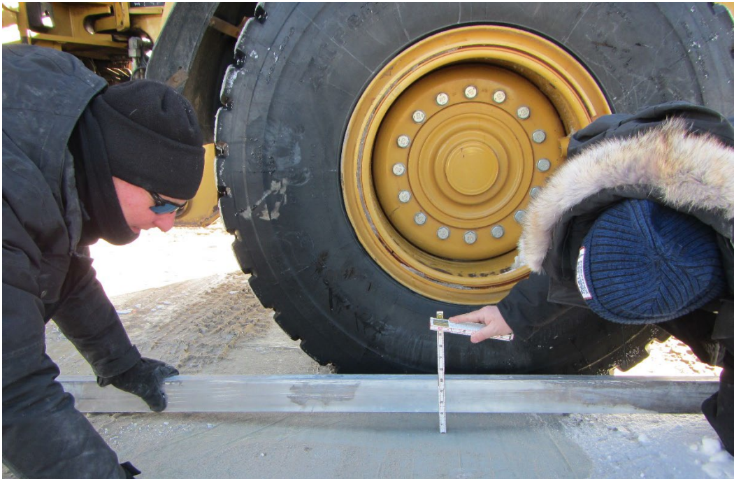
Figure 59. Typical rut depth measurement.
