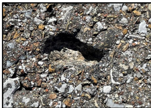
(f) Soft aggregate particle removed with knife
