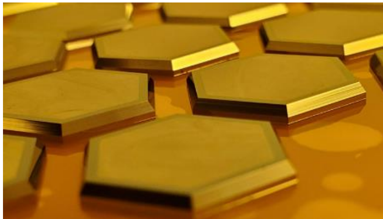
Single DSRD dies ready for stacking
