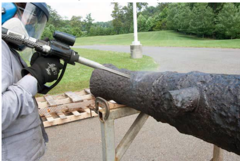
Figure 8. Dry Ice Blasting
