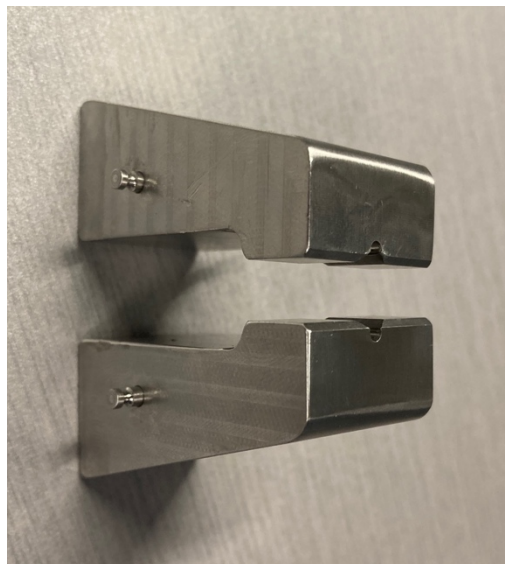
Figure 13. Machined set of grips for torsion testing.
