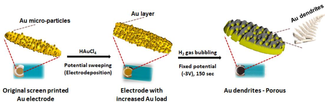
Schematics of the Au screen printed electrode (Au-SPE) modification leading first to the electrochemical deposition of a Au multilayer and then its roughening.
