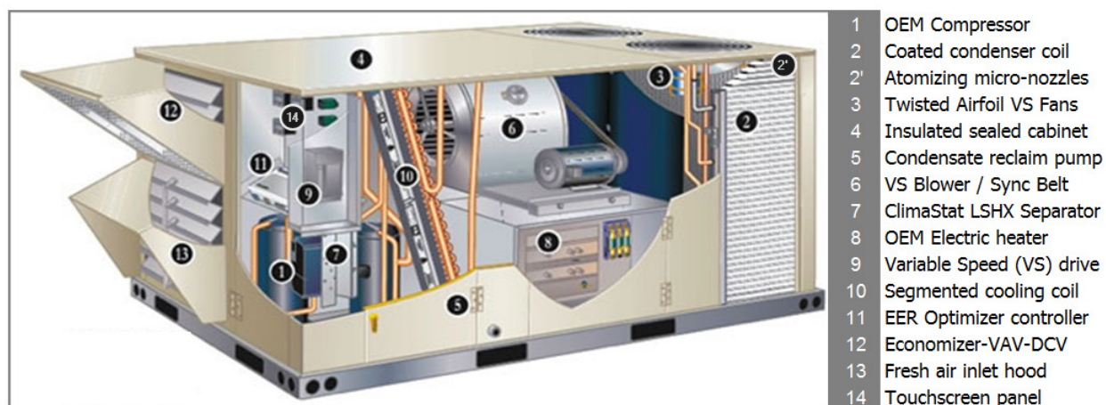
Figure 2. Next Generation Advanced DX Package Unit Component Layout.
