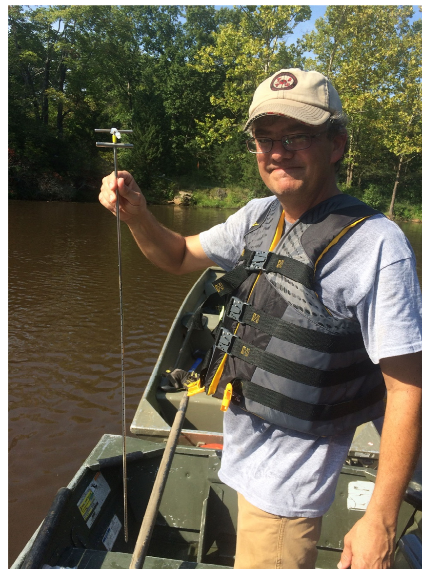
Photo 9: SPME fiber T-Bar sampler
