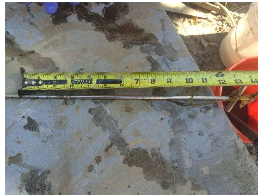
Photo 18: SPME T-Bar sampler ready for processing/sampling
