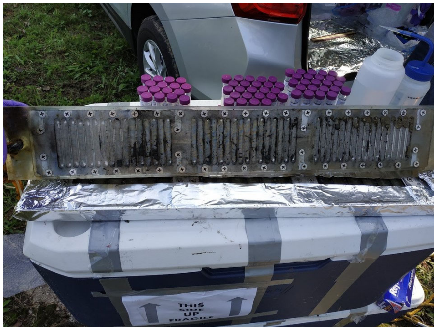
Photo 10: sHRPP just removed from river sediments
