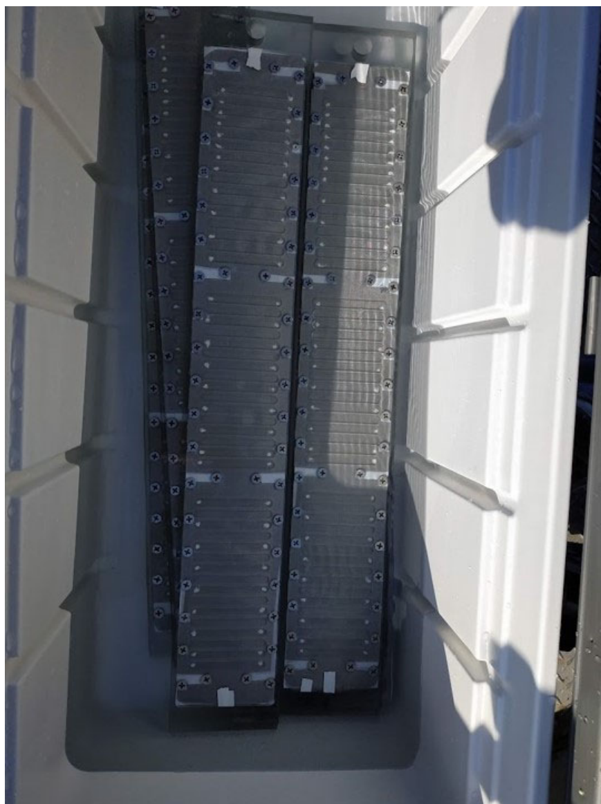
Photo 7: sHRPPs transferred to field site in 100 ppm Br - water
