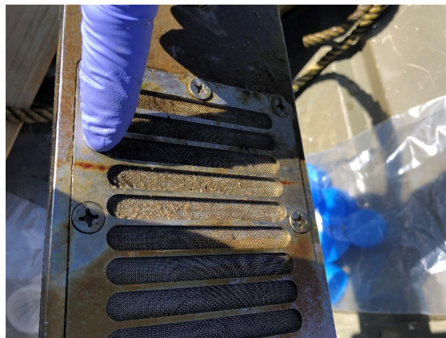
Photo 11: Oxidation indicating sediment-surface water interface
