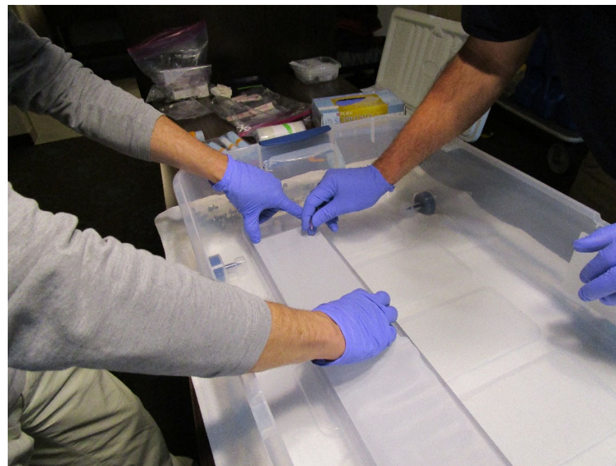
Photo 2: Membranes being installed on sHRPP in 100 ppm Br - water
