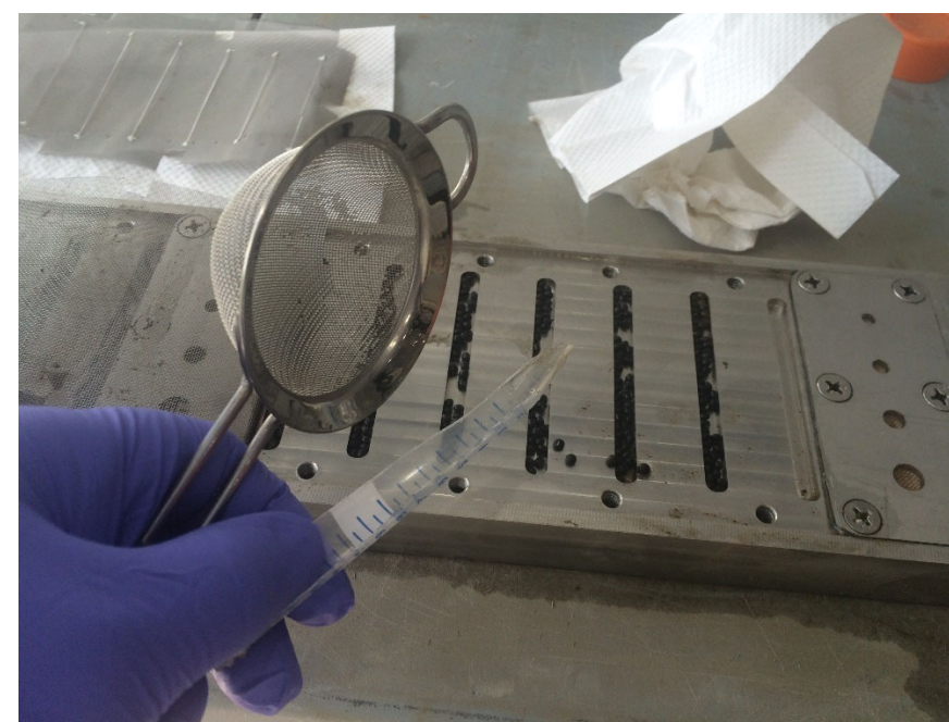
Photo 15: Biosep beads ready for processing/sampling
