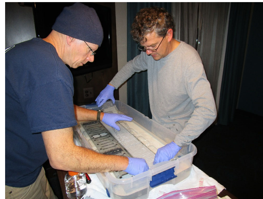
Photo 3: SPME preparation with Biosep beads installed
