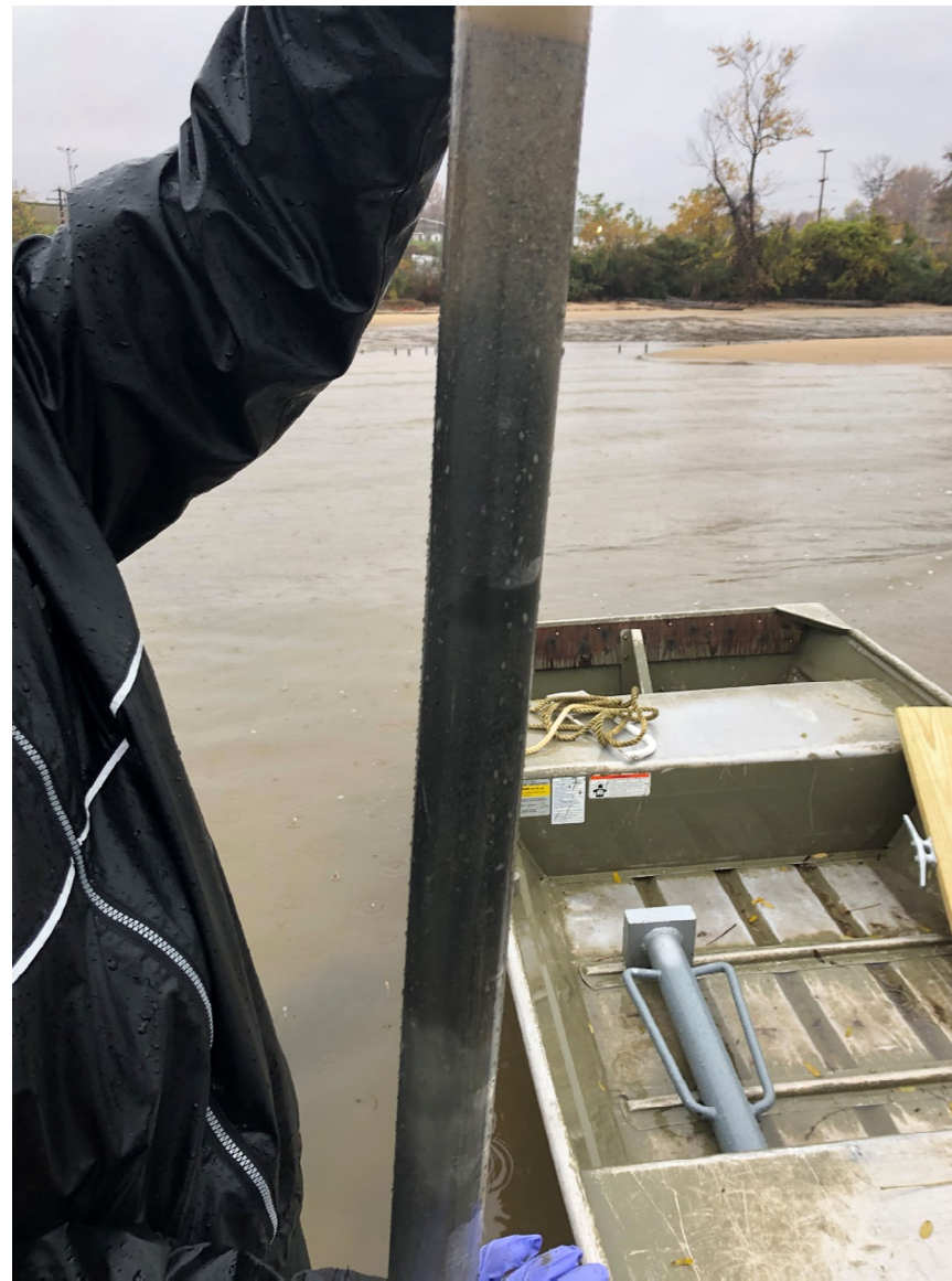
Photo 17: Intact sediment core
