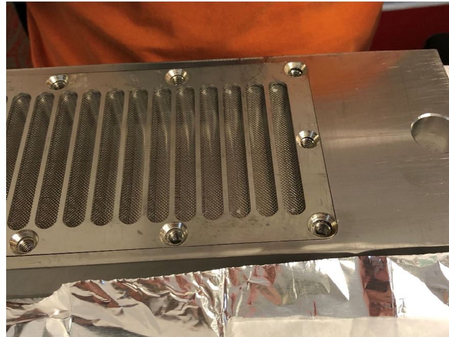
Photo 2: SPME fibers installed on sHRPP
