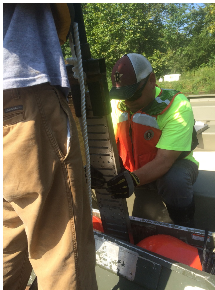
Photo 8: Deployment of sHRPP in creek sediments
