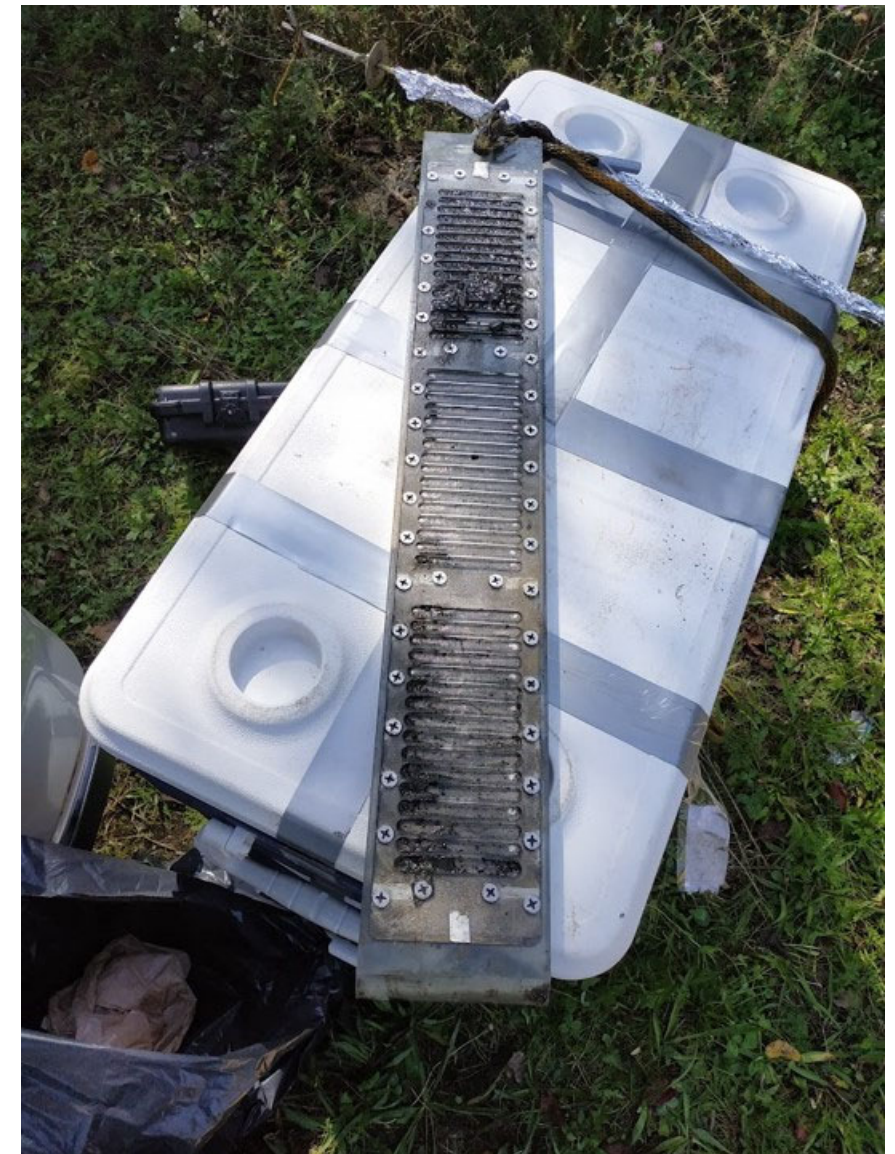
Photo 12: sHRPP and T Bar sampler ready for sampling
