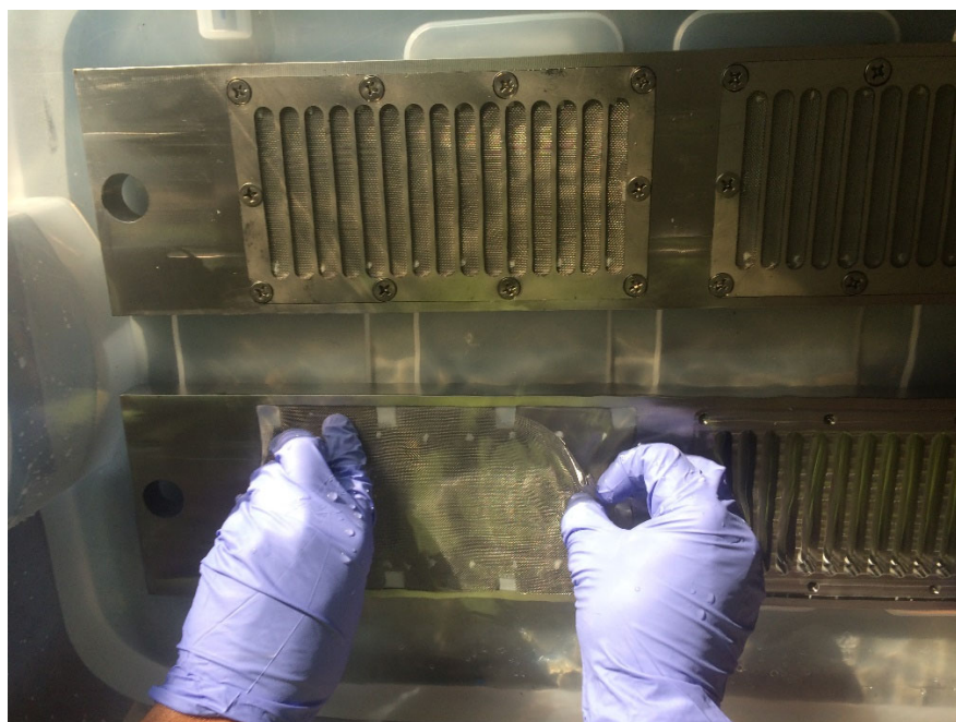
Photo 1: Installing stainless steel mesh over cells in 100 ppm Br - water
