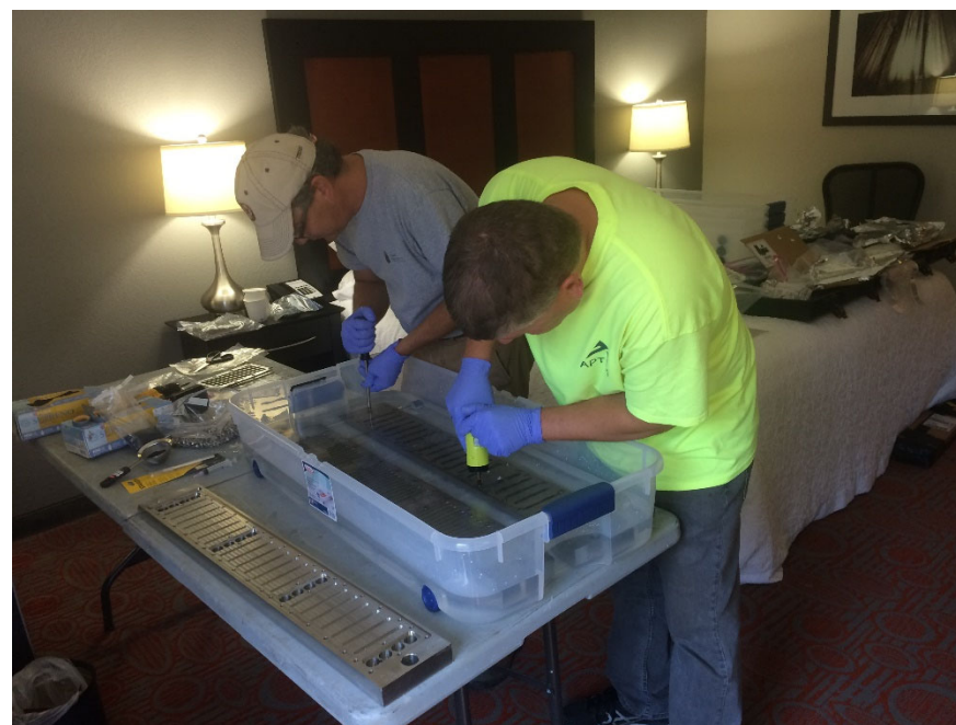
Photo 2: Membrane cover-plates installed in 100 ppm Br - water
