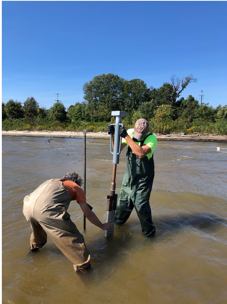
Photo 7: sHRPP deployment into embayment sediments
