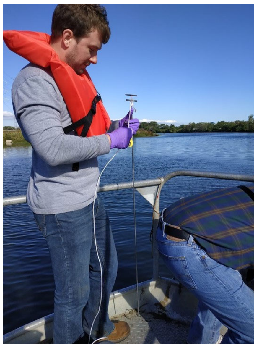
Photo 8: T Bar sampler being prepared for deployment
