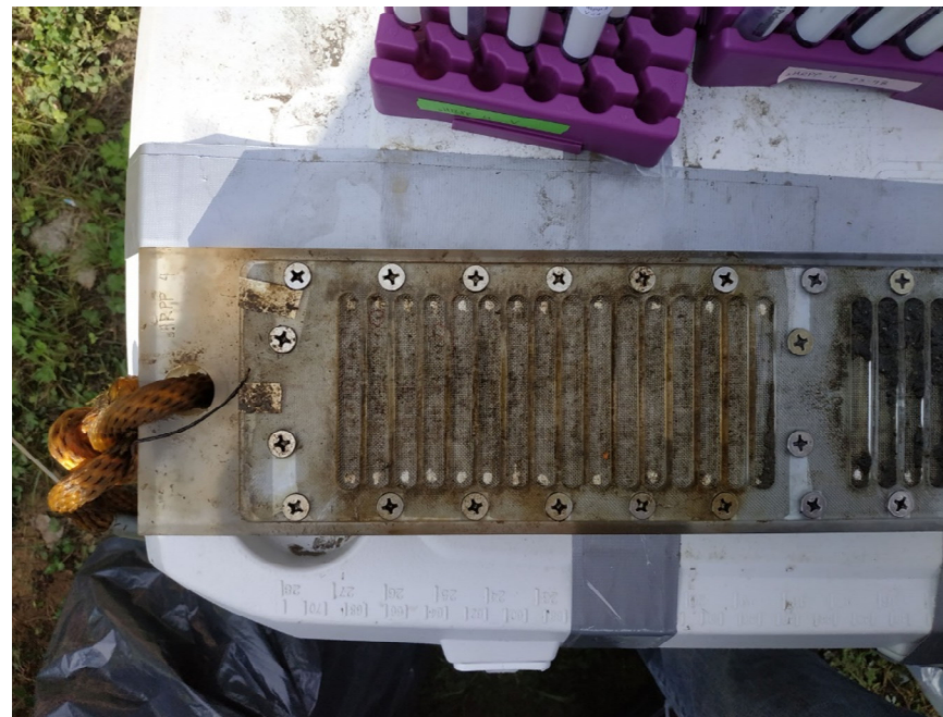
Photo 11: SPME fibers ready for sampling after sHRPP retrieval
