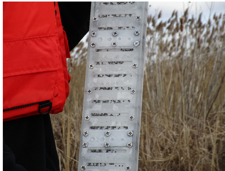
Photo 5: Prepared sHRPP ready for deployment
