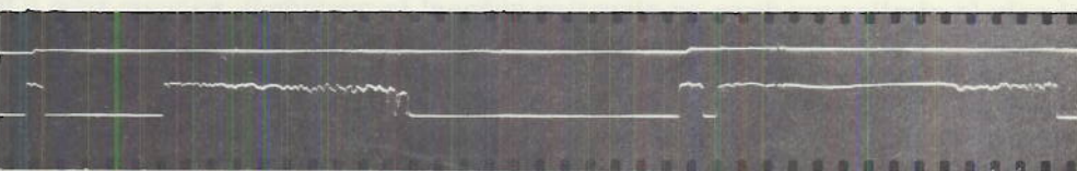
(e) TWO PULSE GROUPS WITH CONTACT BOUNCE—EACH GROUP SAMPLED ONCE. 2.4 15.0 31.5 34.4 3 1.5 39.8 MILLISECONDS
