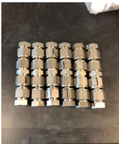
Figure 2.8.1 Reactors and heat source used for hydrothermal reactions. (a) Stainless steel tube reactors used for hydrothermal treatment reactions; (b) Fluidized sand bath used for heating reactors.
