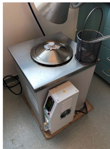
Figure 2.8.1 Reactors and heat source used for hydrothermal reactions. (a) Stainless steel tube reactors used for hydrothermal treatment reactions; (b) Fluidized sand bath used for heating reactors.
