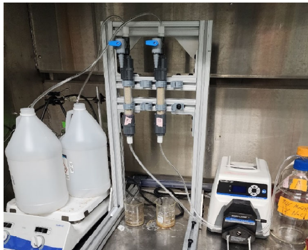
Figure 2.7.1. Photograph of the continuous-flow regeneration apparatus.
