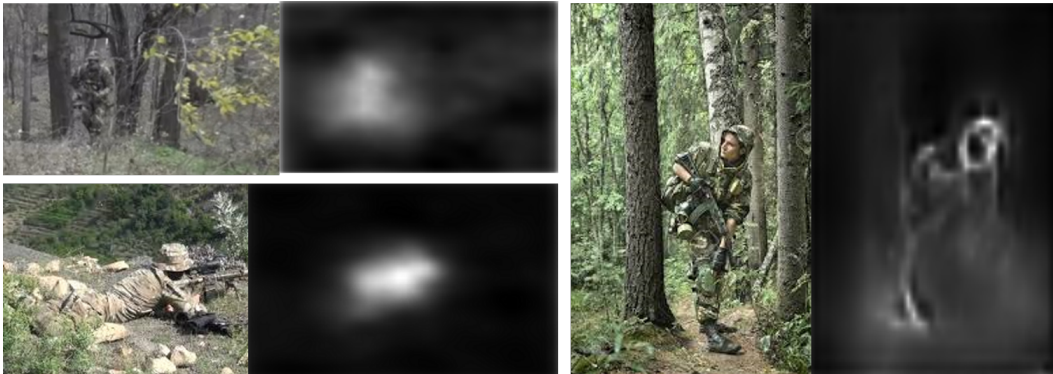
Figure 5: Phase 2 results from trained SINet model applied on previously untrained/unseen camouflaged Marine. In each paired image, the left panel shows the camouflaged Marine while the right panel finds the location of the detected target.
