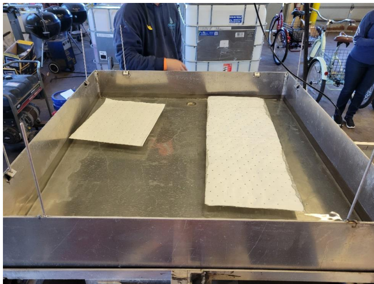
Figure 20. Water-only uptake test with Imbibiter Fiber™ and Oil-Only Heavyweight Pads.
