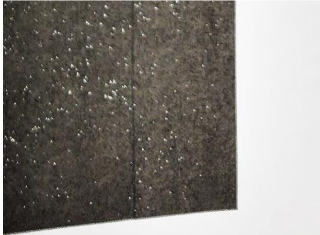
Figure 25. Close view of Imbiber Beads® released from Imbiber Fiber™ after minimal handling. White beads are shown distributed on black paper.
