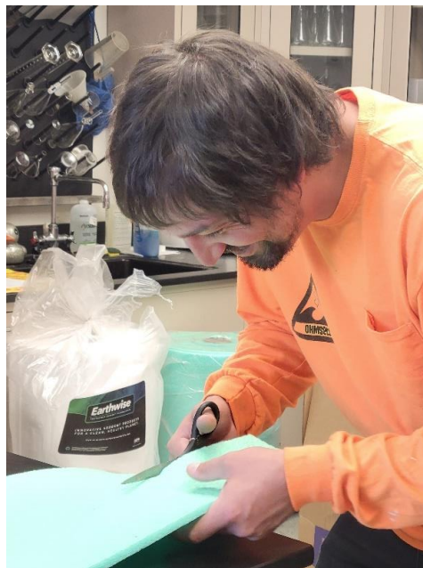
Figure 5. Cutting sorbent sample to proper ASTM size (13 cm x 13 cm).
