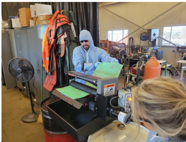
Figure 10. AquaFlex® sorbent sample tested for reusability performance.
