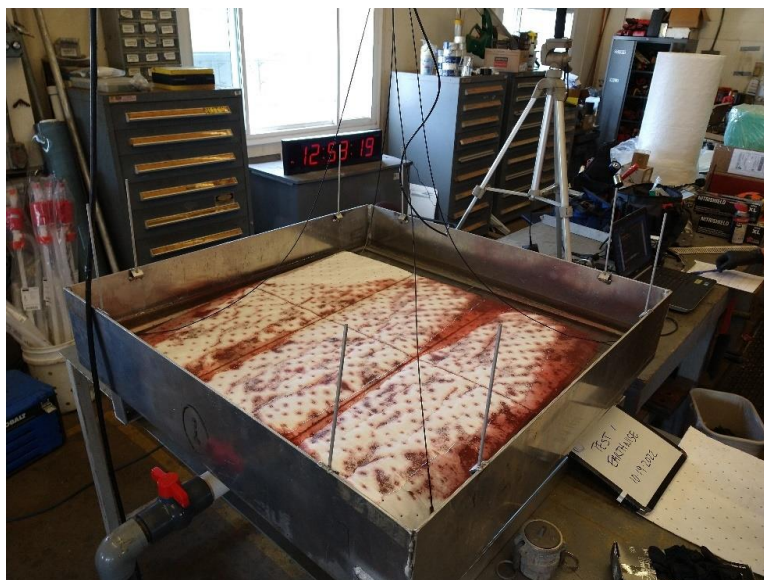
Figure 16. Oil-Only Heavyweight Pads in static conditions during a water uptake test.
