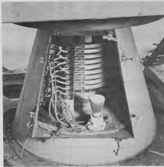
Figure 6 - Slip rings on pedestal shaft
