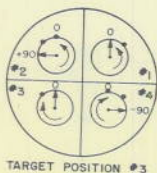
Figure 13 - Phase relation- ship of electrical outputs of the four quadrants
