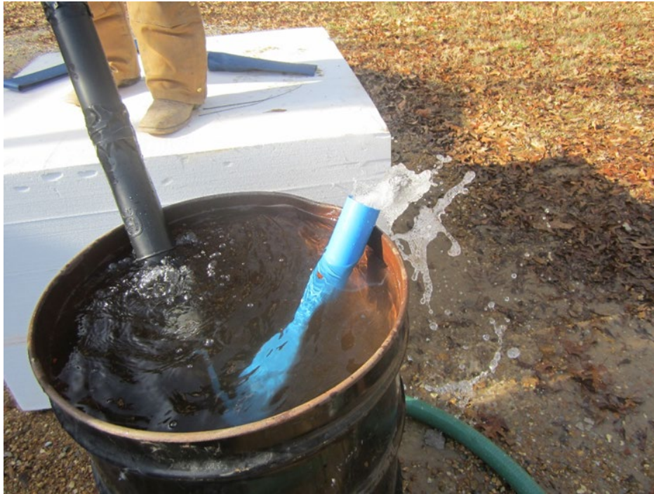
Figure 3. Operation of prototype backpack blower venturi pump.
