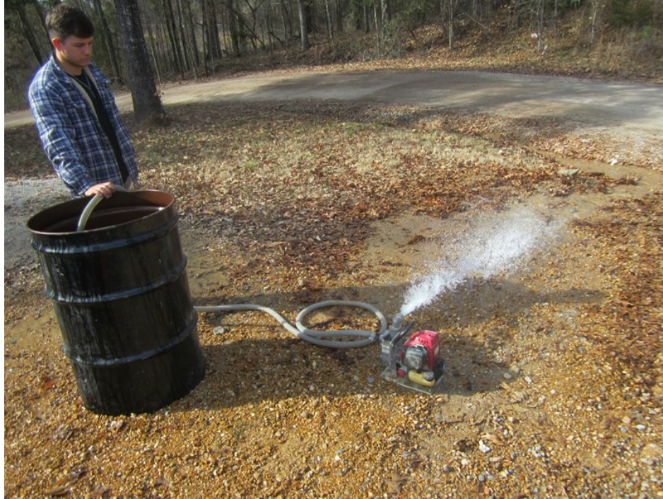
Figure 5. Operation of a Honda WX10 pump.
