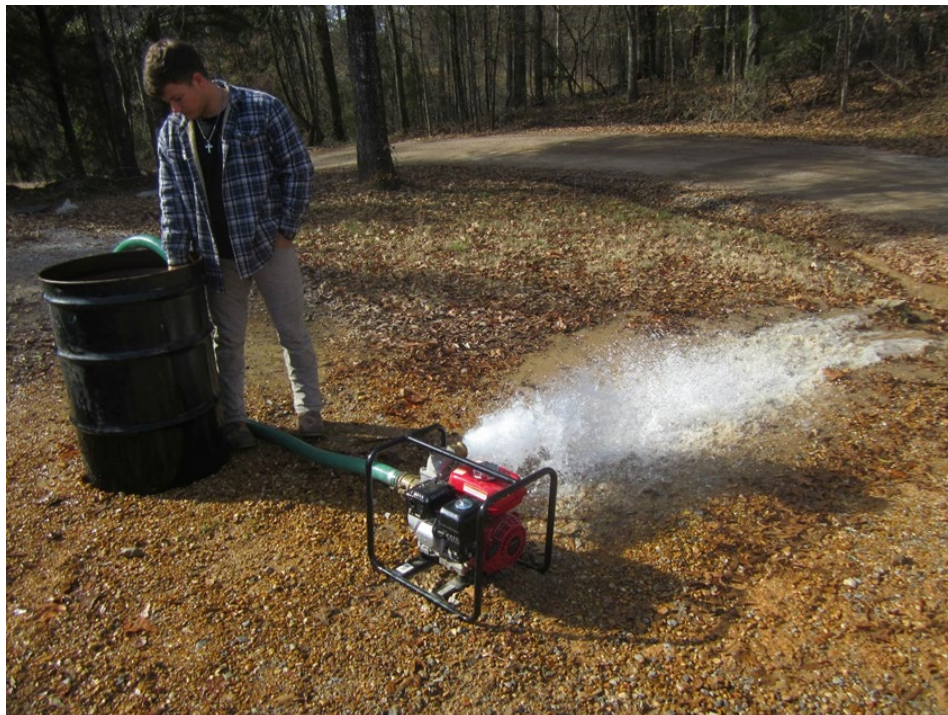
Figure 6. Operation of a Honda WB20XT3 pump.
