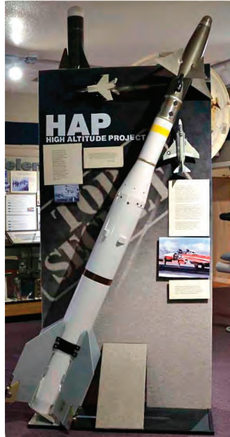
HAP missile model on display at China Lake Museum of Armament and Technology. Note 8-inch-diameter Sparrow motor and 5-inch-diameter Sidewinder front end.
