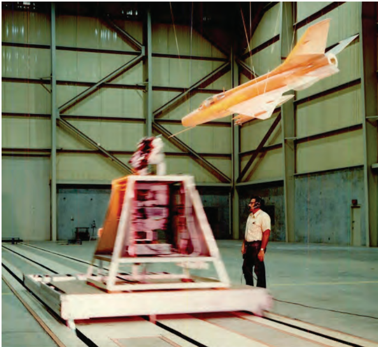
Modeling fuze/aircraft encounter in NWC's Encounter Simulation Laboratory at Corona. Published in D503 Encounter Simulation Laboratory , 1976.
