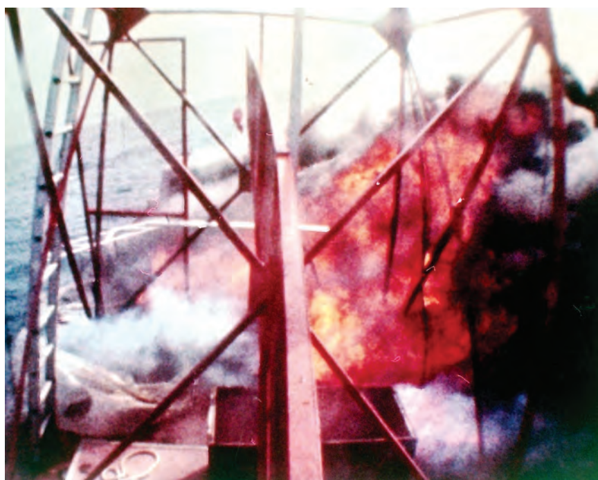
Harpoon impacting (above) and detonating (below) inside QST-35 Seaborne Powered Target (SEPTAR).
