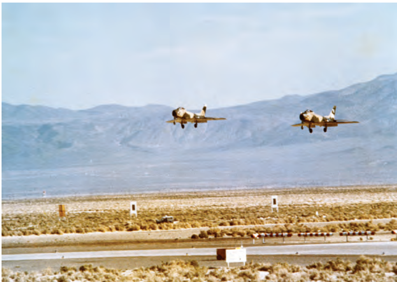
First QF-86H target drone NOLO flight (left) with manned F-86G chase plane (right). Photo courtesy of Gary Verver.
