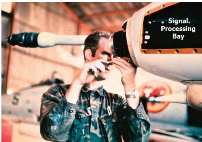
Engineer Gary Ozunas installing Laser Spot Tracker on A-4.
