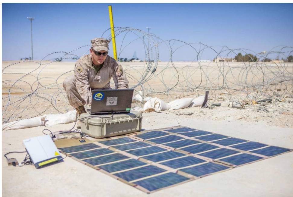
Figure 19. U.S. Marine using a SPACES kit to power a communications system at King Faisal Air Base in Jordan (Marine Corps photo by Sgt. Christopher Q. Stone).
