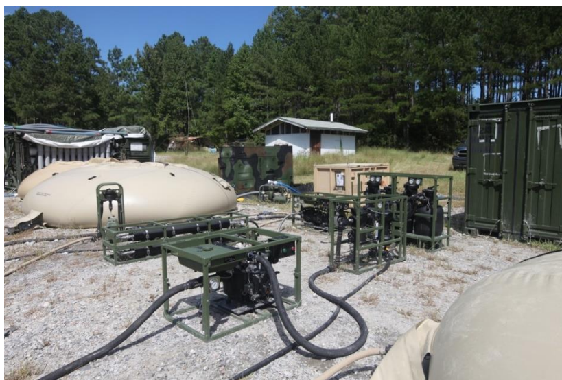
Figure 5. A Lightweight Water Purification System (LWPS) operating at Fort Pickett, VA (U.S. Marine Corps photo by Sgt. Kyle N. Runnels).
