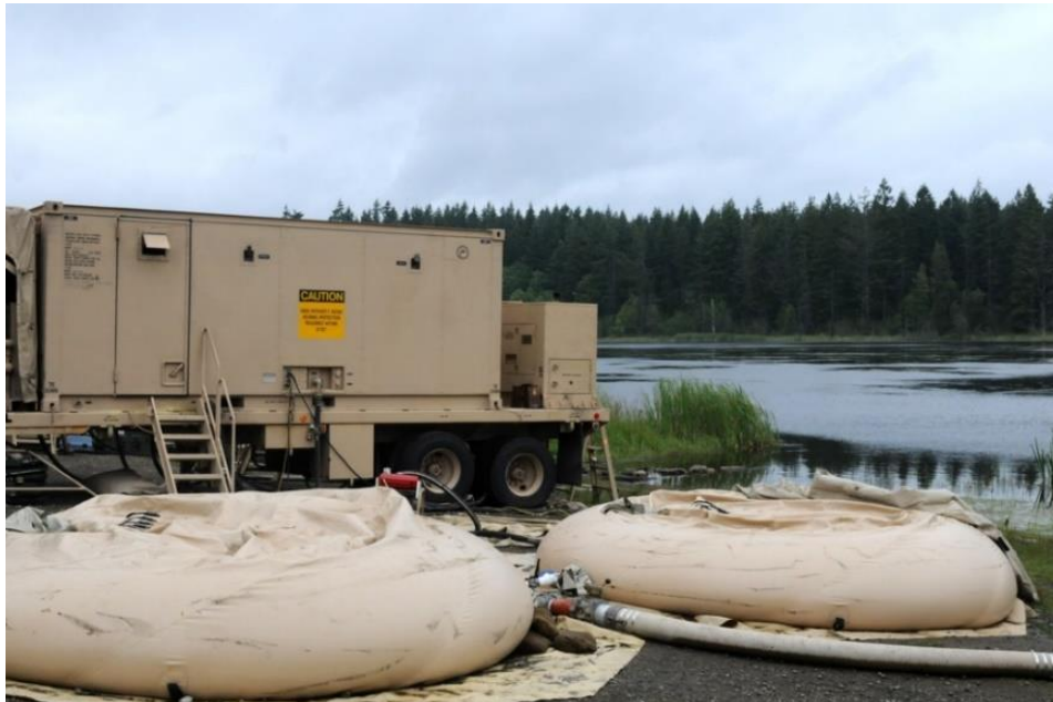
Figure 3. A Reverse Osmosis Water Purification Unit, ROWPU, processing lake water to potable water (filling bladders in the foreground) at Joint Base Lewis-McChord, Washington (US Army photo by Spc. Thomas X. Crough/Released).
