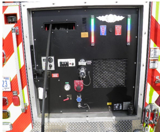
Figure-8: RIV UHP Pump and Foam Control Panel
