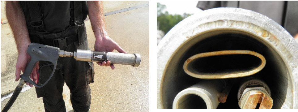
Figure-7: UHP Handline Nozzle & Selected Foam Delivery Spreader Tip Position
