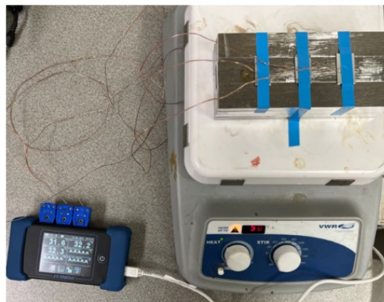
Figure 17. Thermocouple test apparatus and measurement set up
