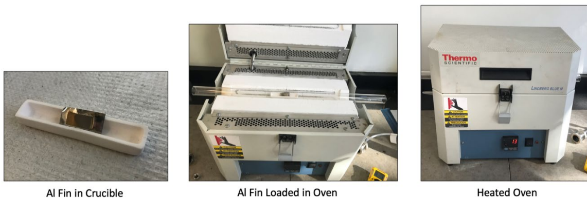
Figure 14. Annealing crucible with sample and oven
