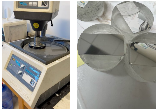
Figure 11. Buehler Ecomet 4 set up (left), and the polished aluminum sample ready to be anodized (right)
