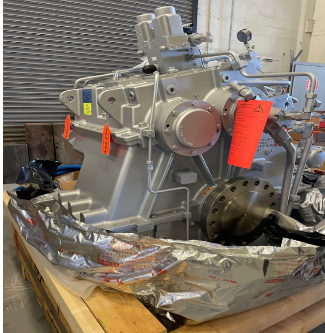
Figure 16. Main Reduction Gear of YTT-11 in workshop for Overhaul and Reinstallation
