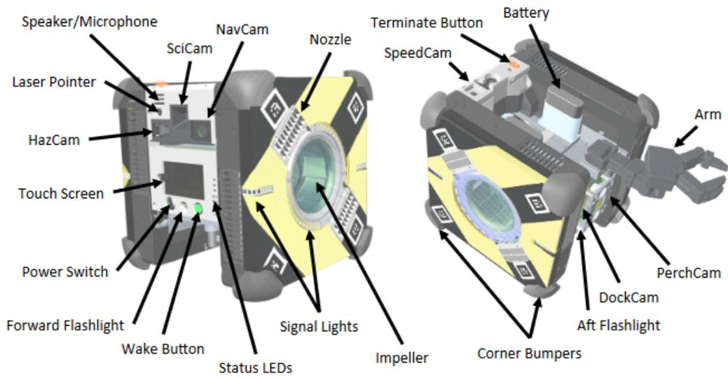
Figure 4. An Astrobeer robot. Source: [6].
