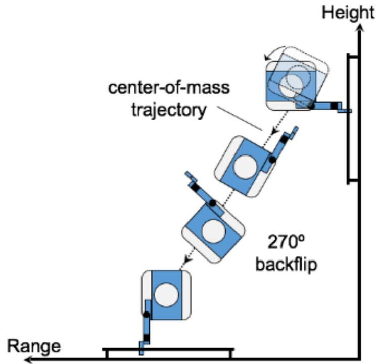
Figure 10. Schematic of Astrobee self-toss maneuver. Source: [20].
