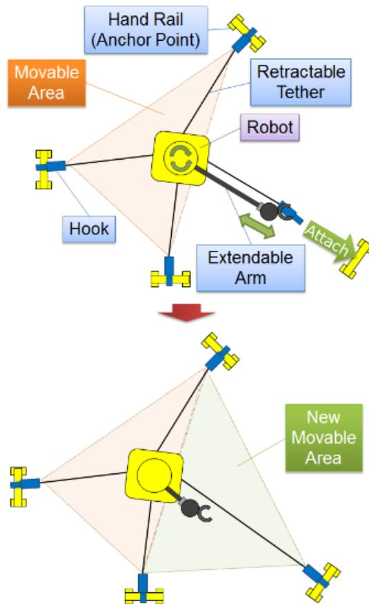
Figure 27. Self-reconfigurable tether-based locomotion concept. Source: [42].
