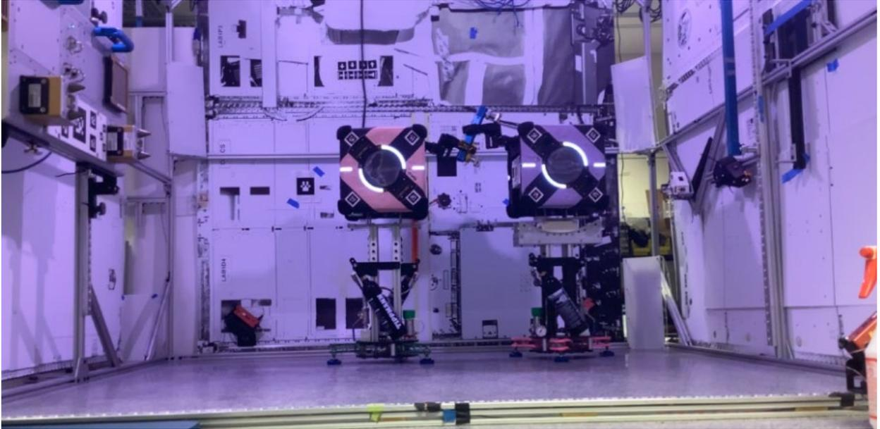
Figure 28. Granite lab with Astrobee simulators
