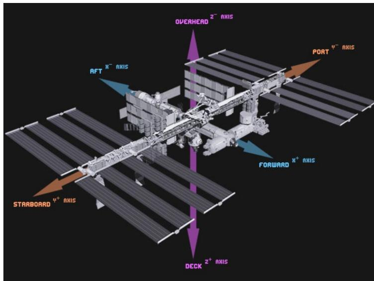
Figure 14. Coordinate system of the ISS. Source: [29].
