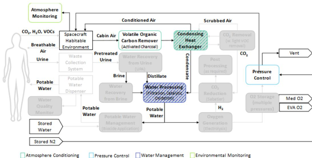
Figure 6. Dormant configuration of the ECLSS. Source: [11].
