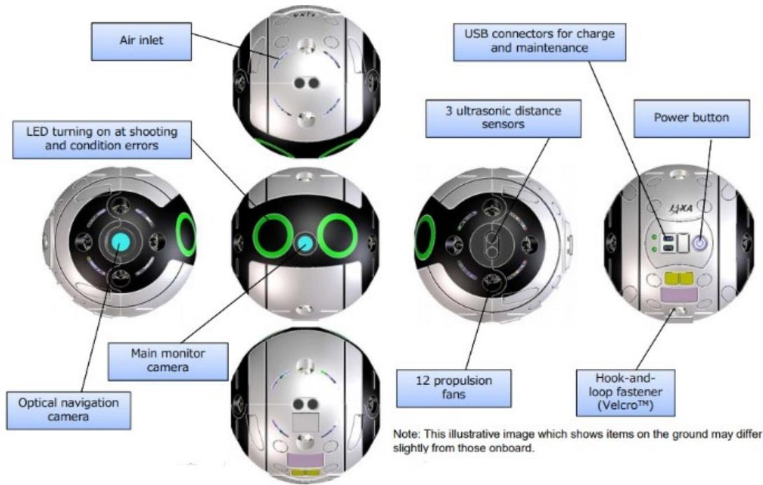
Figure 3. External features of the Int-Ball. Source: [5].
