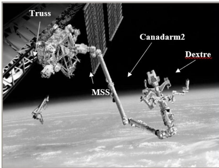
Figure 7. MSS and its subcomponents. Adapted from [12].
