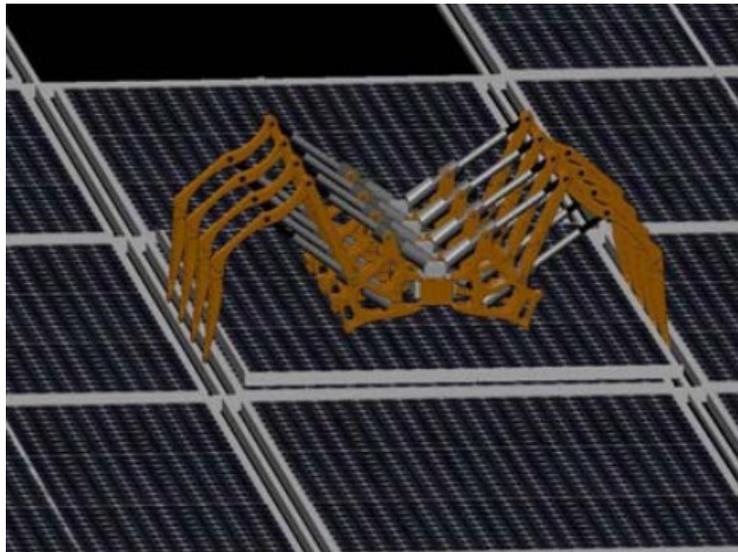
Figure 21. Conceptual arachnid robot moving across a solar array. Source: [34].
