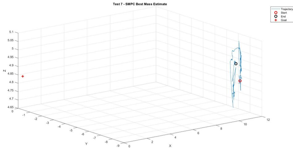
Figure 49. Trajectory of active Astrobees during Test 7
