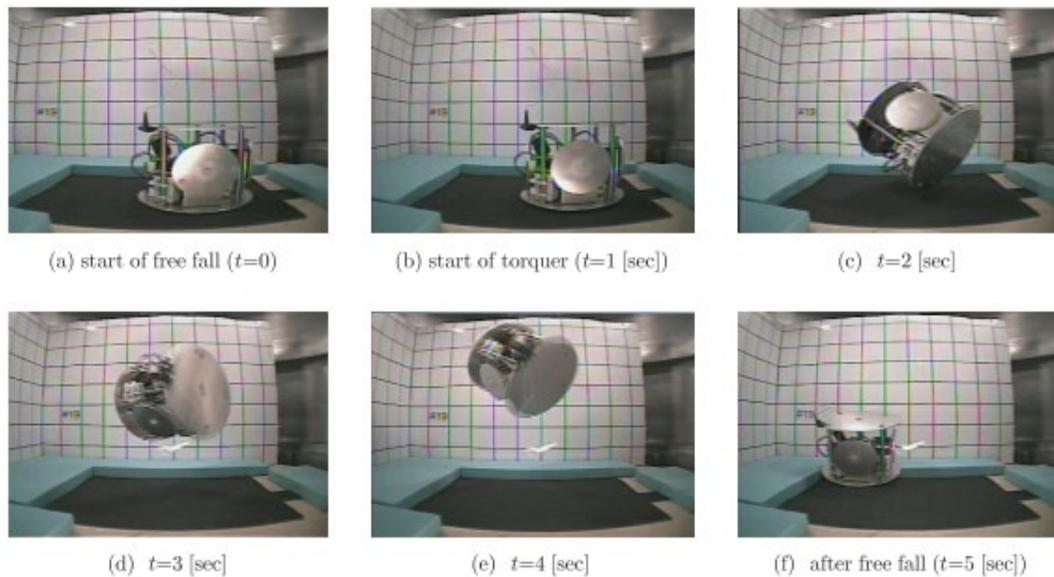
Figure 24. Robot Torquer hopping experiment. Source: [41]
