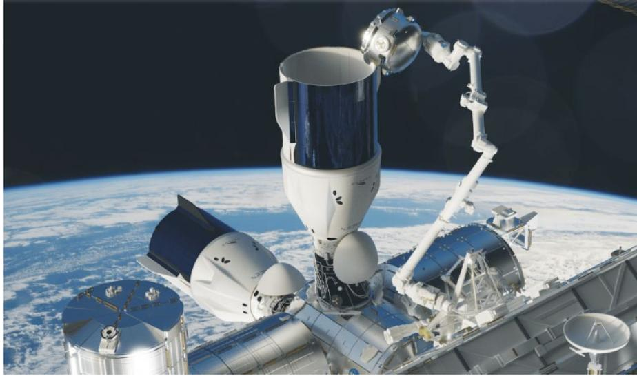
Figure 9. Canadarm2 conducting external cargo offload. Source: [17].
