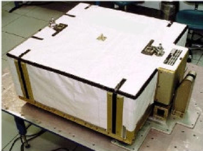
Figure 8. Battery ORU. Source: [12].
