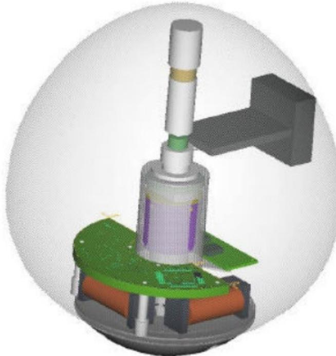
Figure 23. CAD rendering of Fiorini's hopping robot. Source: [39]
