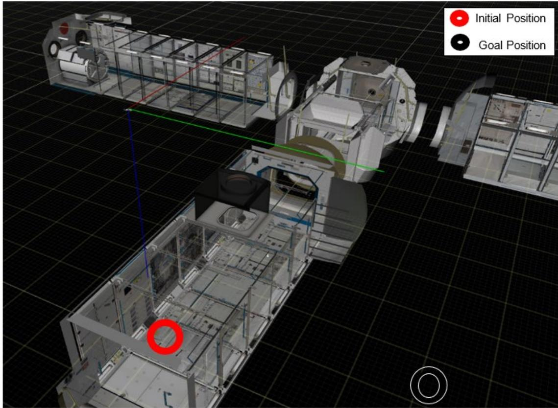
Figure 37. ISS coordinate system. RGB corresponds to XYZ axes. Adapted from [2].
