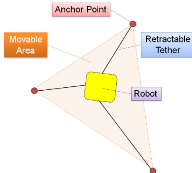
Figure 26. Tether-based locomotion concept. Source: [42].
