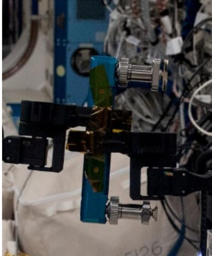
Figure 30. Orientation of perching arm grippers on free floating handrail
