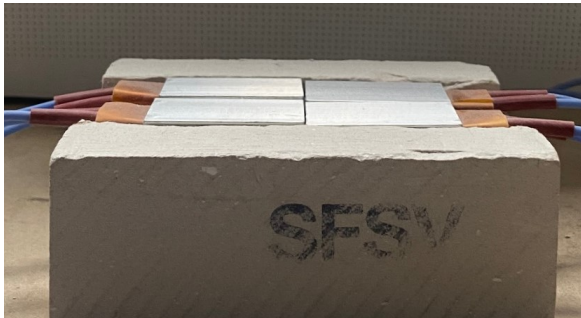
Figure 3.27. Resistance heaters in insulation.
