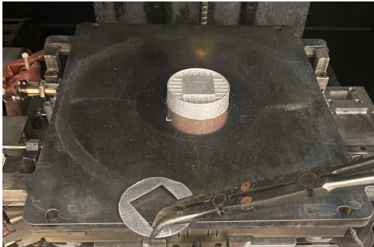
Figure 3.6. Pre-heating the lid (bottom left) prior to installation on the heat sink during printing.
