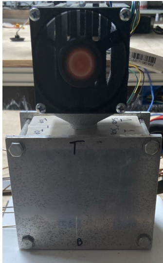
Figure 3.19. Full assembly of thermal conductivity test rig.
