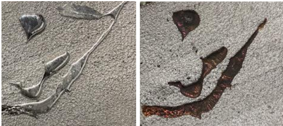
Figure 5.2. Material interaction of FM on Al-4008 substrate before (left) and after (right) heating test.
