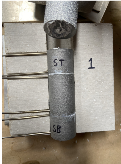
Figure 3.16. Assembling the cylinders and components for the thermal conductivity test, including the application of thermal paste on surfaces.
