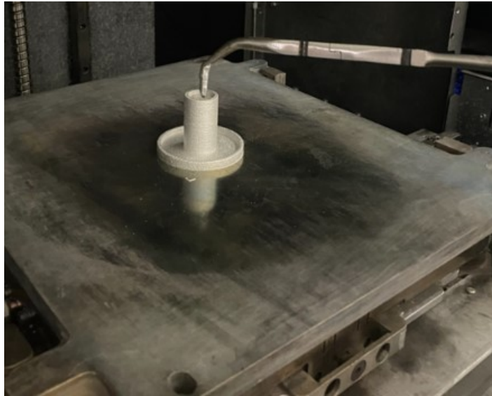
Figure 5.4. Addition of piece of FM ingot into thermal conductivity test cylinder during print.
