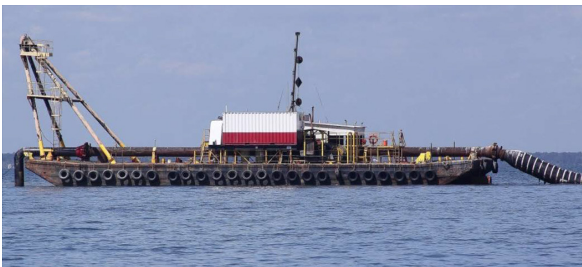
Figure 1.2. Spill Barge Placing Thin Layers of DM in Mobile Bay
