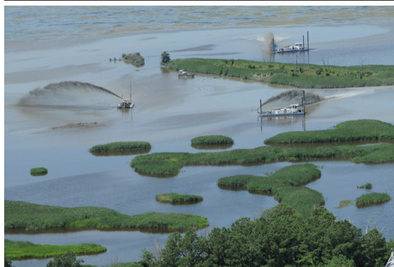
c. Prime Hook, Delaware 12-in (30.48 cm) swinging ladder cutterhead dredge
