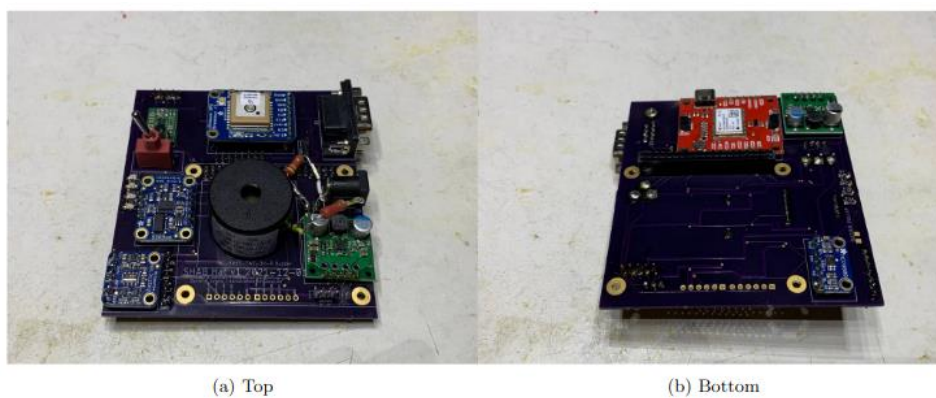
Fig. 1 — SHABHat, custom printed PCB daughterboard for Raspberry Pi with COTS sensors, voltage regulators, and additional parts for autonomous SHAB flights
