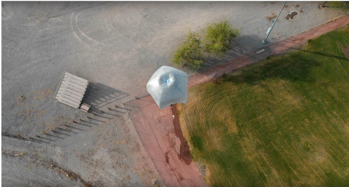
Fig. 3 — Aerial photo of a vented SHAB flight in Tucson with a Styrofoam (EPS) vent mounted to the top of the balloon
