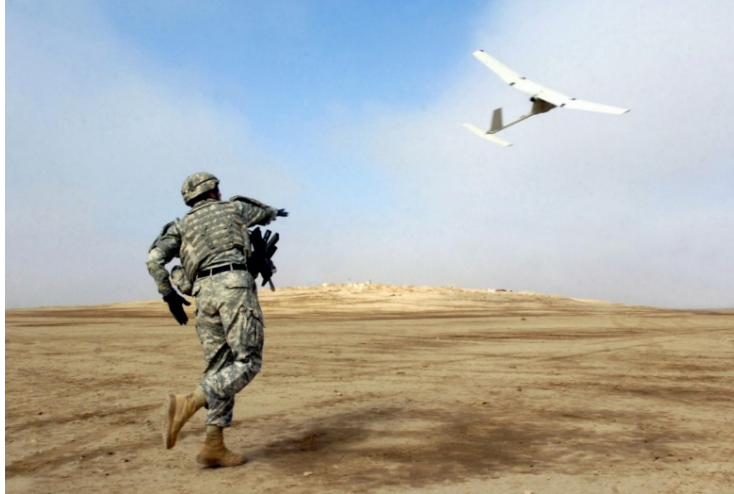
Figure 7. The RQ-11 Raven Group 1 UAS. Source Wikipedia (n.d.a).
