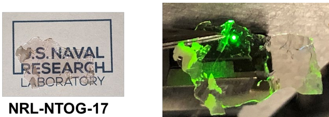
Fig. 7 — Sample of NTOG-17 showing clear pink hue indicating presence of \text{Er}^{3+} (left) and emission of green light when pumped with laser (right).
