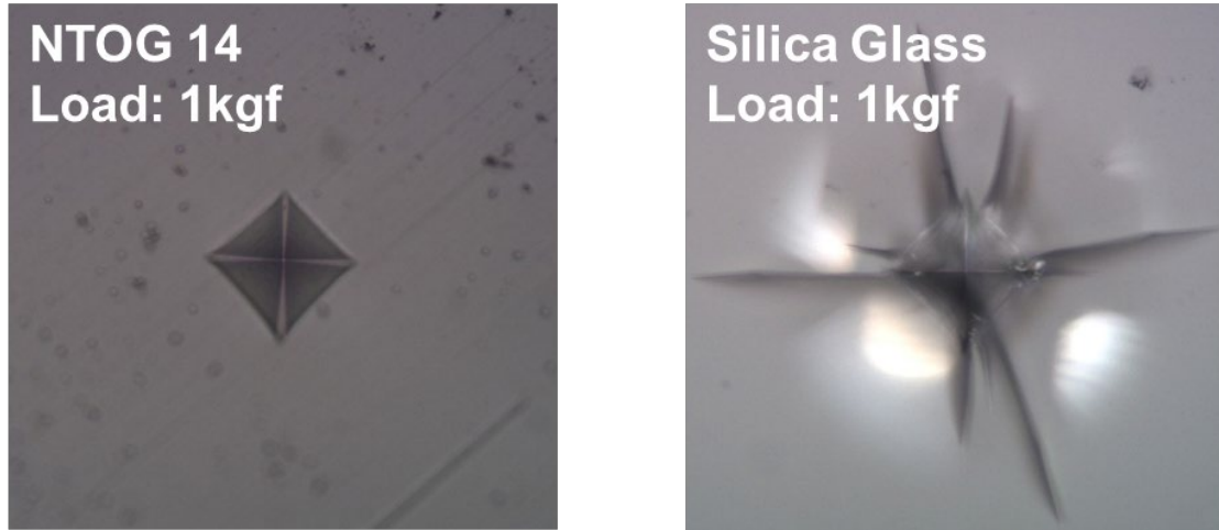
Fig. 3 — Micro-indentation marks comparing NTOGs (no cracking) to regular silica glass when done under high force loads
