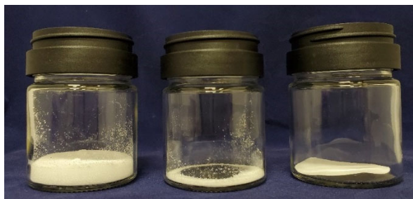
Figure 2: Potassium Chlorate contained within TADDs (L to R: 25g, 2.5g, 20mg printed coupon)
