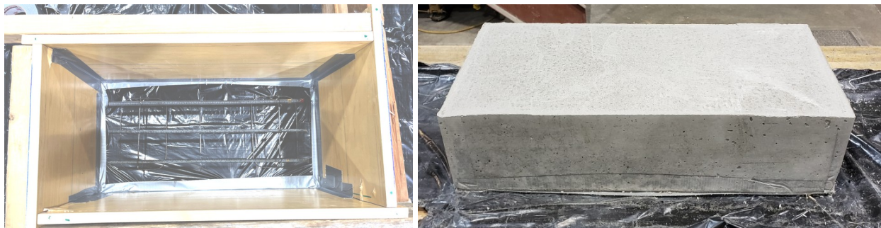
Figure 9: Form for a small concrete block with a rebar grid (left), and completed block that was cast using a mix containing metallic fibers (right).
