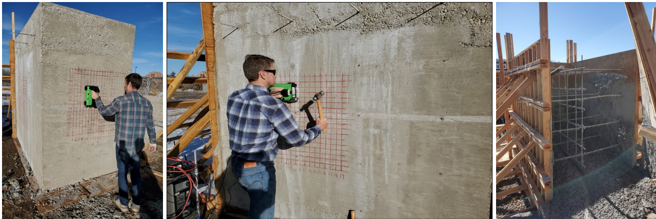
Figure 7: Conducting an GPR scan on a poured block (left), MASW scan (center), and a collapsed form showing internal reinforcements (right).
