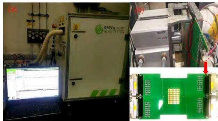
Figure 1. Experimental system: (a) Fuel cell test station; (b) current density distribution tester.
