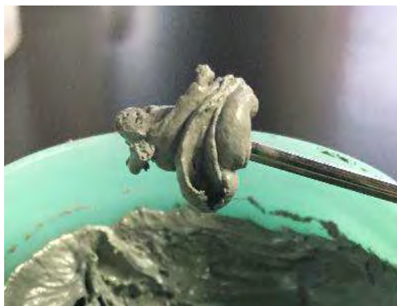
Figure 2. 95%Sn - 5%Sb paste to prepare Sn-based porous layers.
